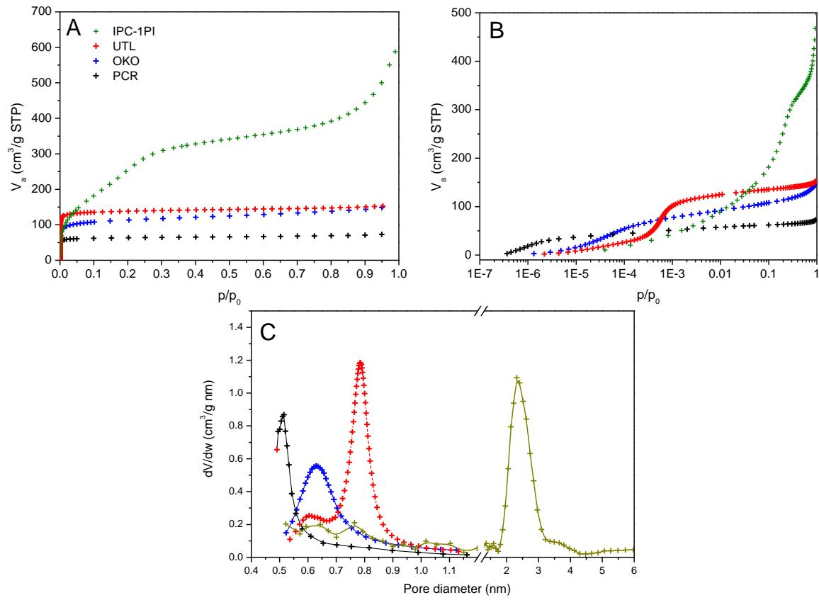
**Fig. SI-1** Argon adsorption isotherms measured at -186°C displayed in linear (A) and semilogarithmic scale (B) and pore-size distribution calculated from the adsorption data by SAEIUS software (C).
