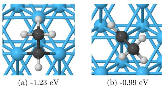
Figure 1: The two geometries found for CH<sub>3</sub>CH. The binding energy for the geometry in (a) is 0.24 eV lower than in (b) and is taken to be the default geometry for CH<sub>3</sub>CH in all other calculations.
