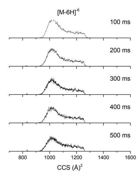
Figure 2. TIMS profiles as a function of the desolvation time for [M-6H]<sup>-6</sup> i-motif DNA.
