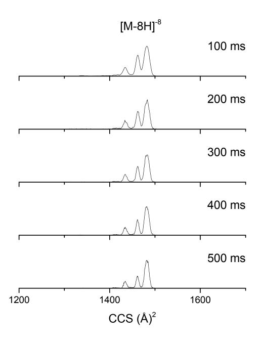
Figure 4. TIMS profiles as a function of the desolvation time for [M-8H]<sup>-8</sup> i-motif DNA.
