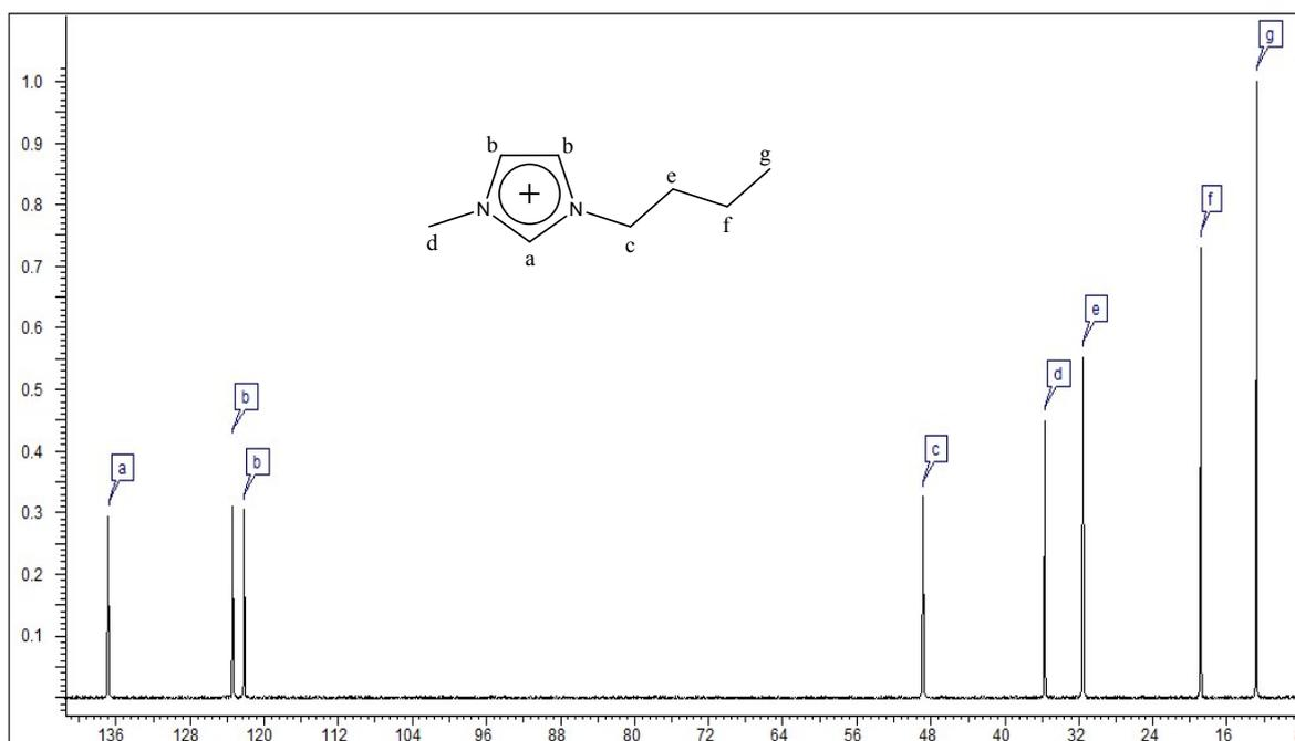
(c)  $^1\text{H}$  NMR spectrum of pure  $[\text{C}_4\text{C}_1\text{im}][\text{N}(\text{CN})_2]$  in neat condition at 200 MHz using  $\text{CDCl}_3$  capillary
