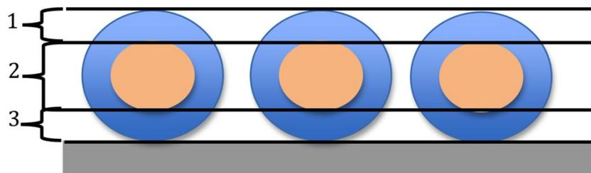
**Figure S10.** Schematic illustration of the model for adsorbed intact micelles on the surface. Three isotropic layers are used to represent the micelles.
