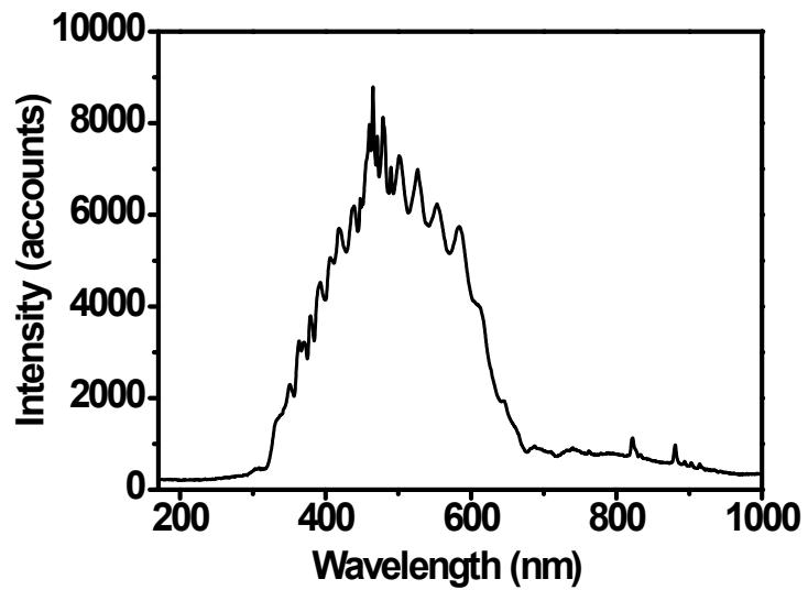
**Fig. S3.** Experimental conditions of  $\text{CH}_4$  photooxidation. a, Setup of the  $\text{CH}_4$  photooxidation. b, The spectrum of the Xe lamp.
