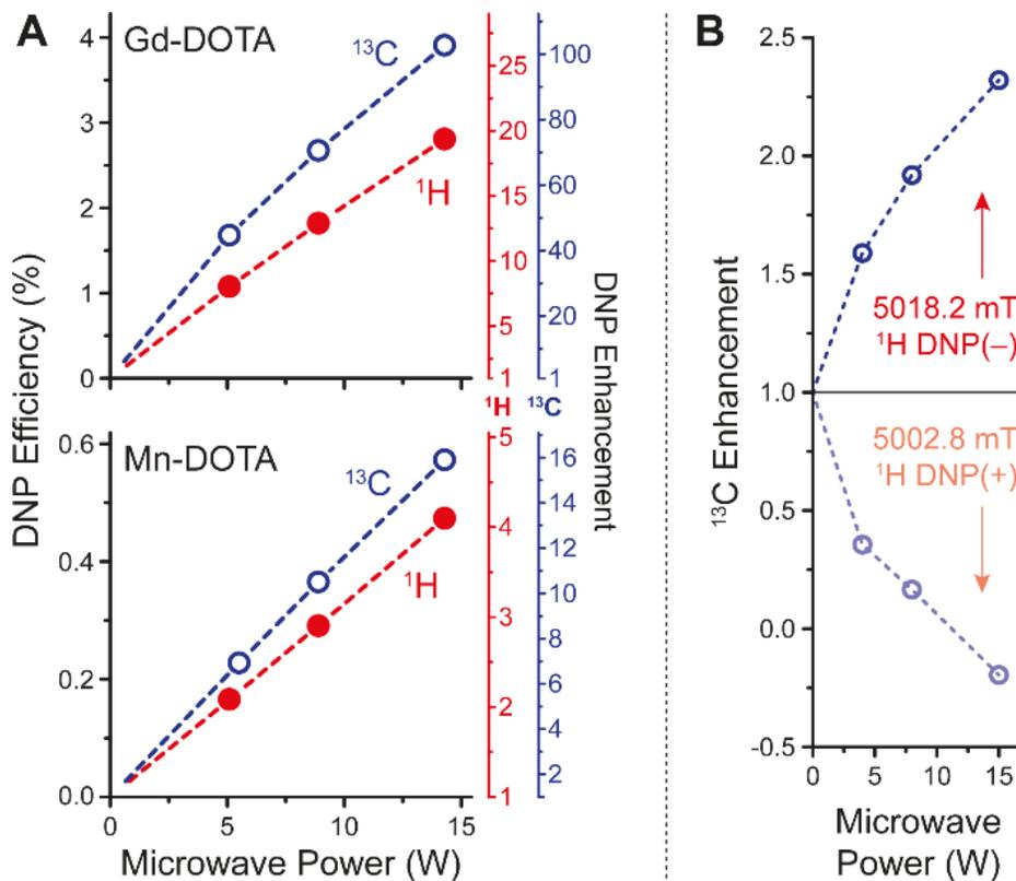
**Figure S1.** (A) Power dependence of  $^1\text{H}$  (full circles, red) and  $^{13}\text{C}$  (open circles, blue) DNP with Gd-DOTA. Left abscissa represents DNP efficiency relative to the theoretical maximum for each nucleus; right abscissas are  $^1\text{H}$  (red) and  $^{13}\text{C}$  (blue) enhancement factors. (B) Power dependence of “indirect”  $^{13}\text{C}$  enhancement at optimum (positive or negative)  $^1\text{H}$  enhancement.
