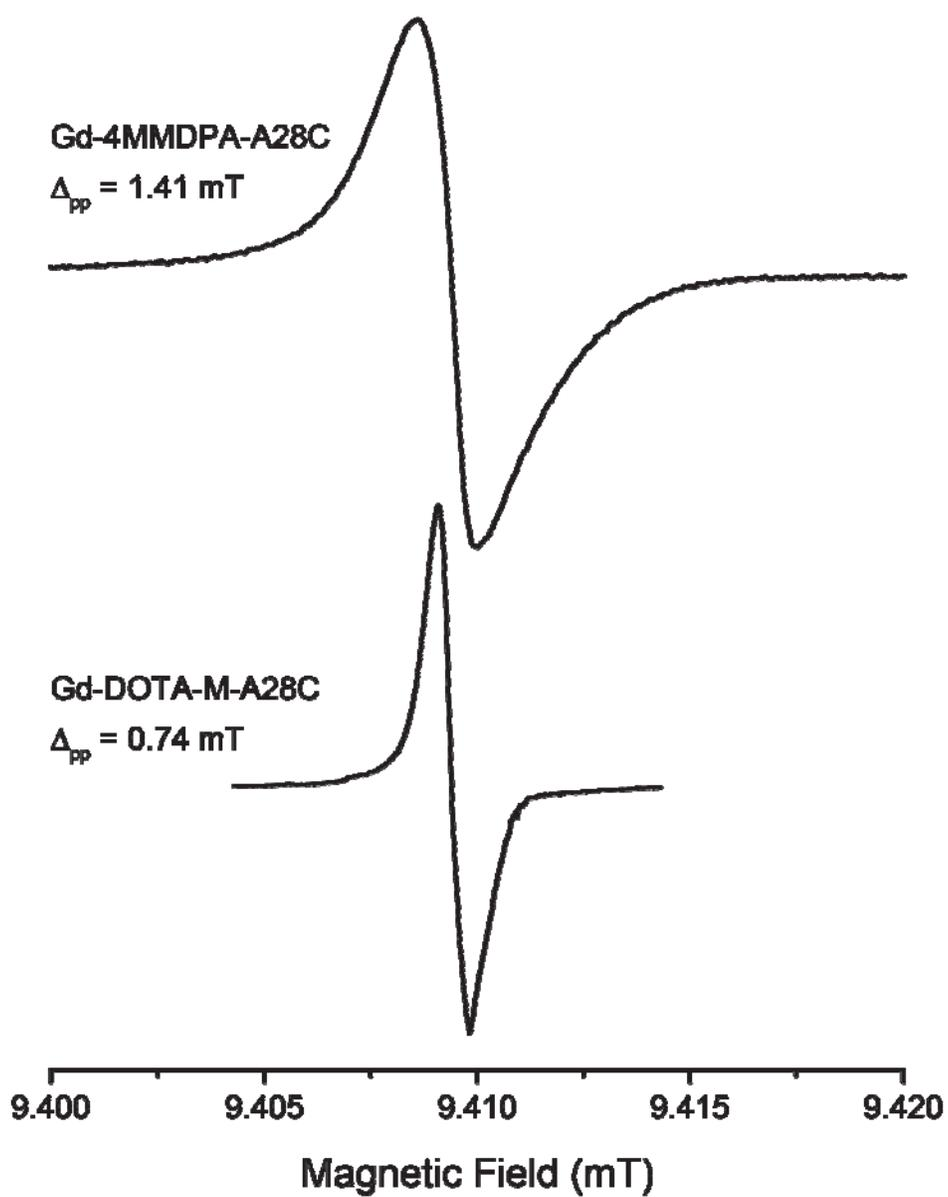
**Figure S4.** Cw EPR spectra of frozen DNP-solutions of Gd-4MMDPA-labeled and Gd-DOTA-M-labeled A28C mutant of ubiquitin measured at a  $\mu\text{w}$  frequency of 263 GHz and a temperature of 100 K.  $\Delta_{pp}$  is the peak-to-peak linewidth of the cw spectra (*i.e.*, first derivative of the absorption spectra).
