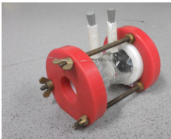
Figure 5: Picture of the transference cell. The electrodes are housed in an inner Teflon ring (white) and an outer PVC ring (red) used to press the electrodes against the glass container.
