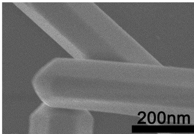
Figure 1A High-magnification FESEM image of the Te NWs.
