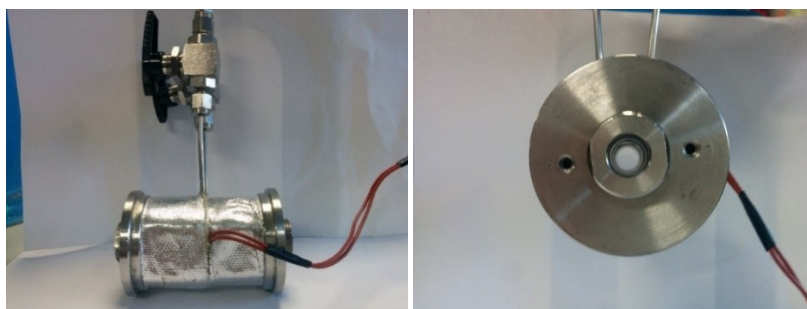
Fig. S8 The photo of high-pressure UV-Vis instrument for measuring the Kamlet-Taft parameters (instrument length: 9 cm; volume, diameter and length of the cuvette are 2.3 ml, 1.2 cm, 2.0 cm, respectively)
