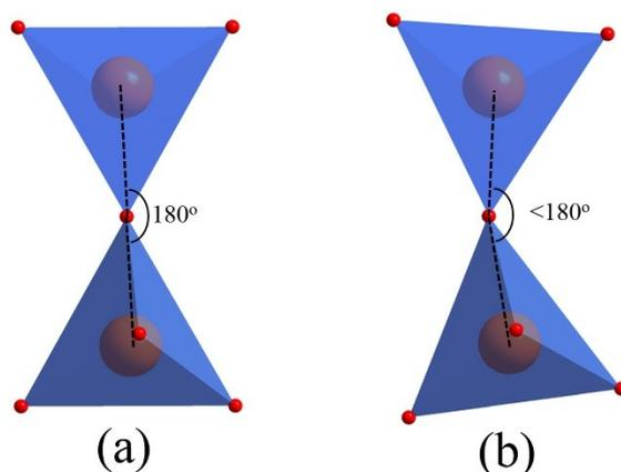
Fig. S3 The schematic V-O-V bond angle in  $\text{ZrV}_2\text{O}_7$  normal structure (a) and superstructure (b).
