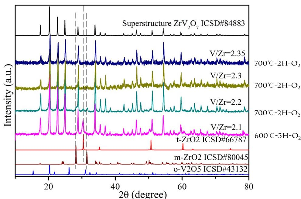
Fig. S1 XRD patterns of synthesized samples with different V/Zr ratio and annealing temperature.
