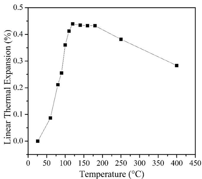
Fig. S4 Linear thermal expansion of superstructure  $ZrV_2O_7$  nanofibres in the temperature range of RT~400°C
