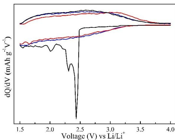
Fig. S5 CV curves of  $ZrV_2O_7$  nanofibres electrode at a voltage window of 1.5~4 V vs.  $Li/Li^+$ .
