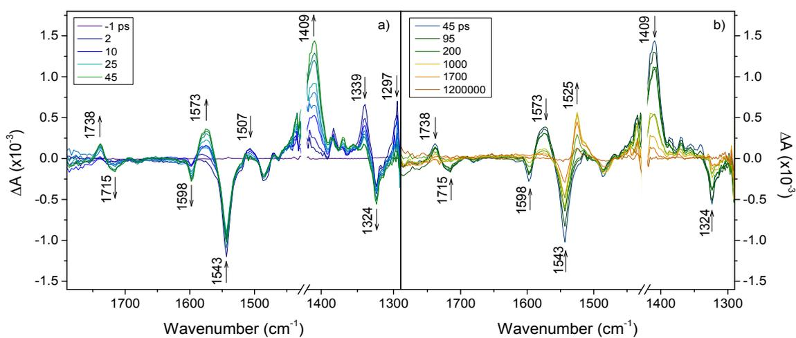
**Figure S5** TRIR spectra of **2** in  $\text{CH}_2\text{Cl}_2$  at early (a) and late (b) times after excitation. Region of the spectra not shown between 1440-20  $\text{cm}^{-1}$  due to absorption by the solvent.
