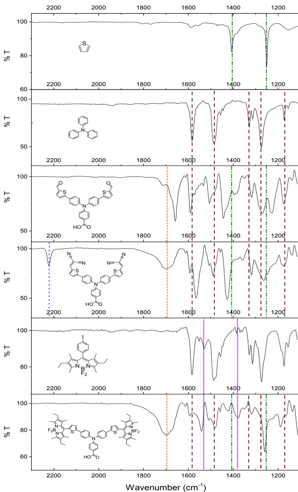
**Figure S2.** Ground state ATR FTIR spectra of **1**, **2** and their corresponding precursor molecules. The corresponding assignments of the vibrational bands are shown; phenyl bands (dashed lines), carbonyl bands (short
