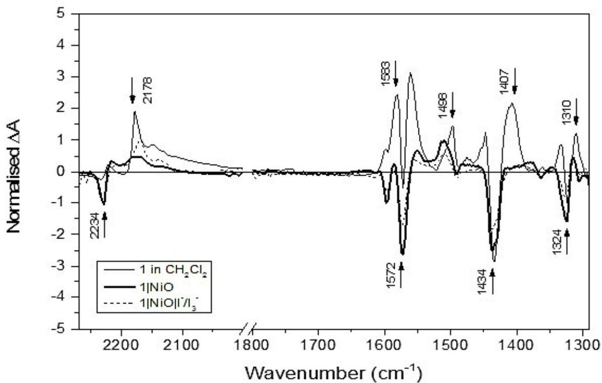
**Figure S4.** Overlay of the TRIR spectra of **1** in  $\text{CH}_2\text{Cl}_2$  (thin solid black),  $1|\text{NiO}$  (thick solid black) and  $1|\text{NiO}|I_3^-$  (dashed black) at a delay time of 15 ps after excitation at 532 nm.
