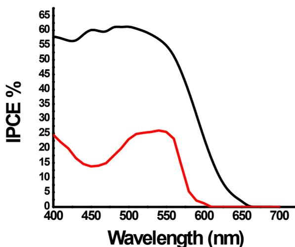
**Figure S1.** Spectral response of p-DSCs incorporating **1** (black) and **2** (red). The cells were assembled as described in reference <sup>21</sup>.
