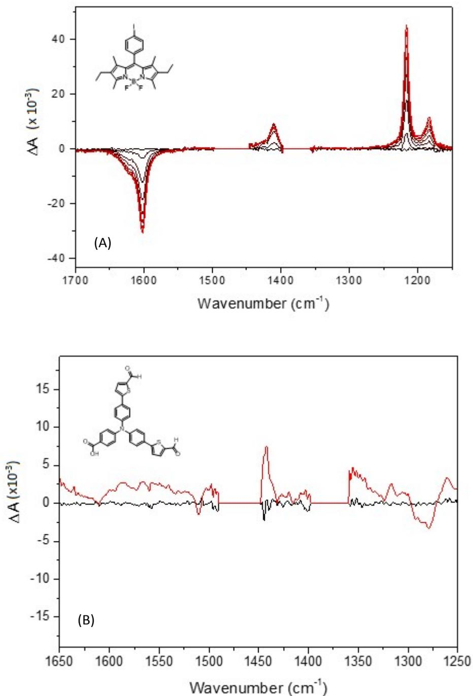
**Figure S8** (A) Infrared difference spectra of the electrochemical reduction of a bodipy derivative in an electrolyte solution of TBAClO<sub>4</sub> and CDCl<sub>3</sub> at -1.08V vs. Fc<sup>+0</sup>. Solvent signals have been omitted at 1475 and 1375  $\text{cm}^{-1}$ . (B) Infrared difference spectra of triphenylamine derivative before (black) and after (red) applying a positive potential of 0.92V vs. Fc<sup>+0</sup>. Solvent signals have been omitted at 1475 and 1375  $\text{cm}^{-1}$ .
