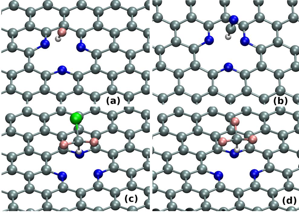
FIG. 4. DFT-based optimized structures of (a) HF (b) HCN (c)  $\text{CHClF}_2$  and (d)  $\text{CHF}_3$  on top of the defect-site of SV-3N.
