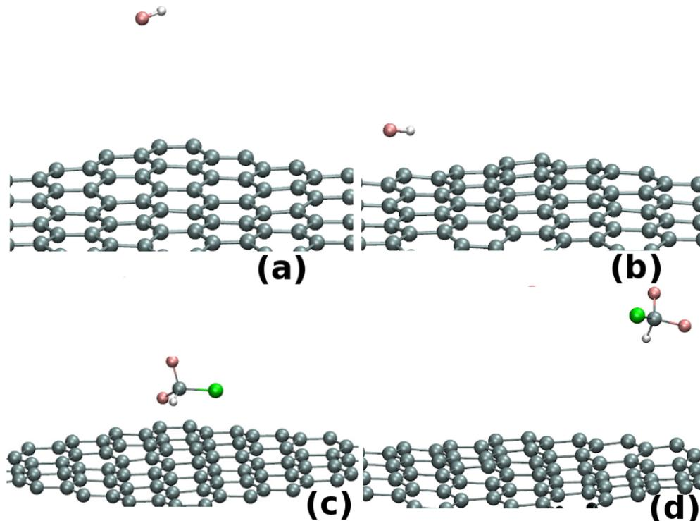
FIG. 2. Snapshots of (a,b) HF and (c,d)  $\text{CHClF}_2$  on top of pristine graphene. BOMD simulations are performed in 300 K; snapshots are captured at (a,c) 0.5 ps and (b,d) 6 ps. White, pink and green colored balls represent hydrogen, fluorine and chlorine, respectively.
