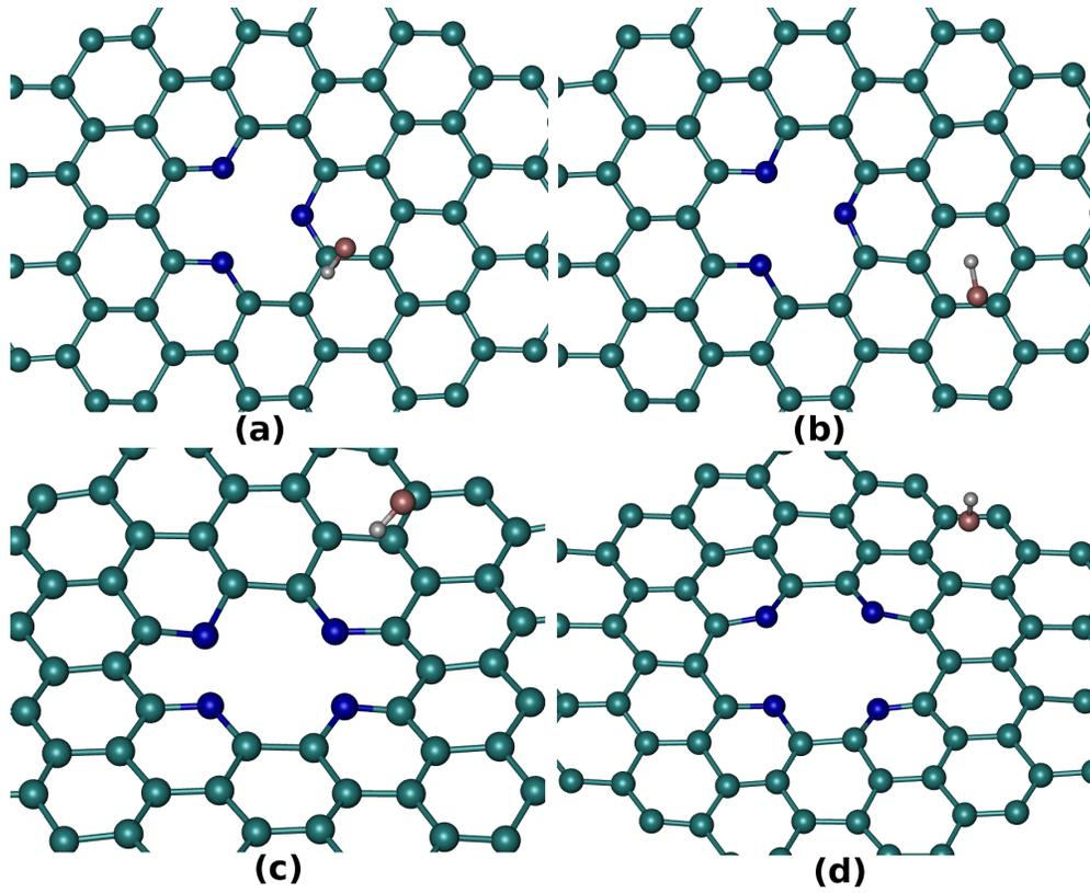
FIG. 8. Snapshots of configurations of HF on SV-3N at 600 K after (a) 4ps (b)4.2 ps and on DV-4N at 650 K after (c) 2ps (d) 2.1 ps BOMD simulations.
