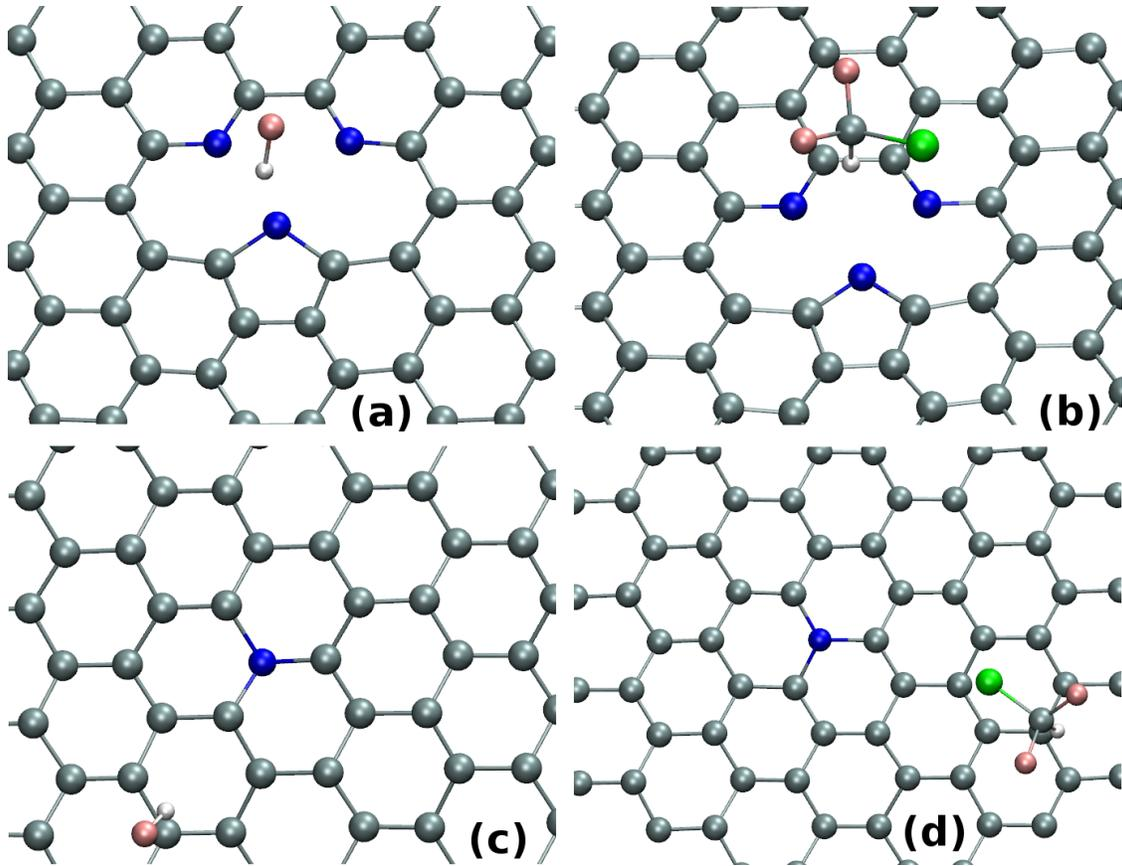
FIG. 3. Various snapshots of configurations of (a) HF and (b)  $\text{CHClF}_2$  trapped on defect-site of pyrrolic nitrogen doped sheets after 10ps BOMD simulation are shown. Snapshots of (c) HF and (d)  $\text{CHClF}_2$  on graphitic nitrogen doped sheets after 10 are given.
