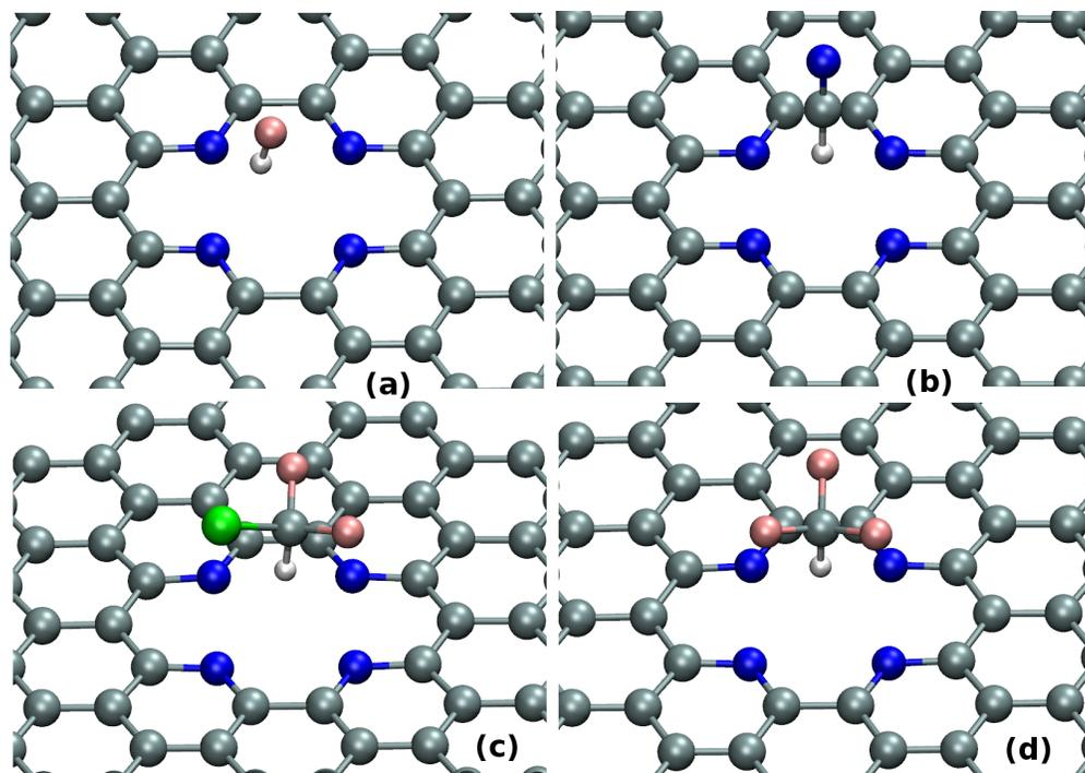
FIG. 5. DFT-based optimized structures of (a) HF (b) HCN (c)  $\text{CHClF}_2$  and (d)  $\text{CHF}_3$  on top of the defect-site of DV-4N.
