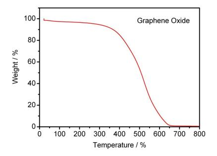
2. Figure S1. TGA of graphene oxide (GO) in oxygen at a rate of 10 °C min<sup>-1</sup>.
