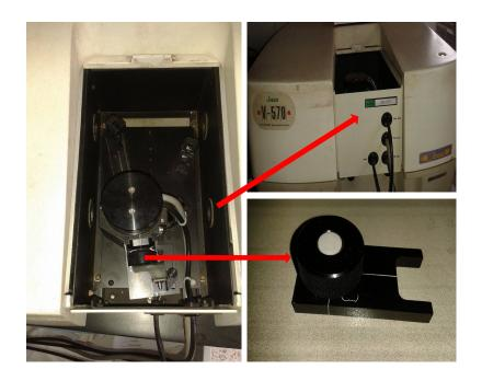
S1: The integrated sphere unit in the UV-Vis-NIR-scanning spectrophotometer (JASCO V-570 spectrophotometer, Japan)
