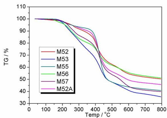
**Fig. S4.** Temperature-dependent TG curves of dyes.
