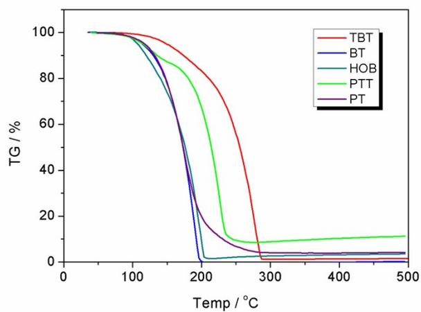
**Fig. S3.** Temperature-dependent TG curves of different donor units. Clearly, **TBT** is more stable than other donor units in terms of thermal stability.
