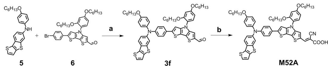
**Scheme S1.** Schematic routes for the M52A dye: (a) *t*-BuONa, Pd<sub>2</sub>(dba)<sub>3</sub>, Xphos, toluene, reflux 8 hours; (b) Piperidine, Cyanoacetic acid, CHCl<sub>3</sub>/CH<sub>3</sub>CN (v/v, 1/2), reflux, 8 hours.
