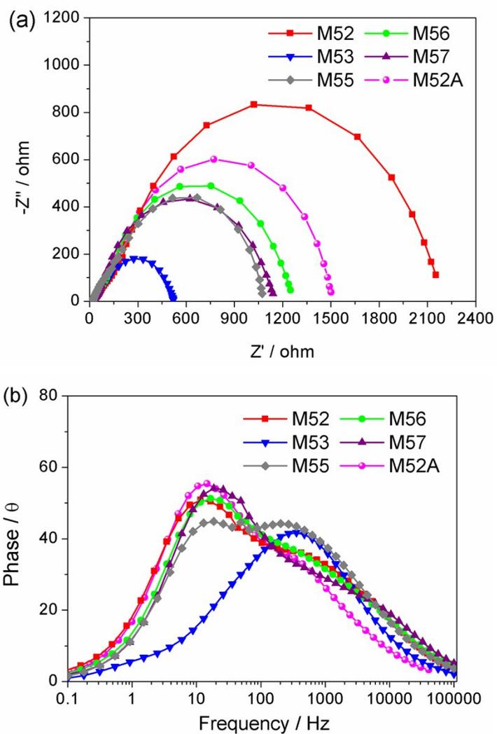
**Fig. S1.** EIS for DSSCs based on the studied dyes measured in the dark under  $-0.8 \text{ V}$  bias displayed in the form of Nyquist plots (a) and Bode phase plots (b).
