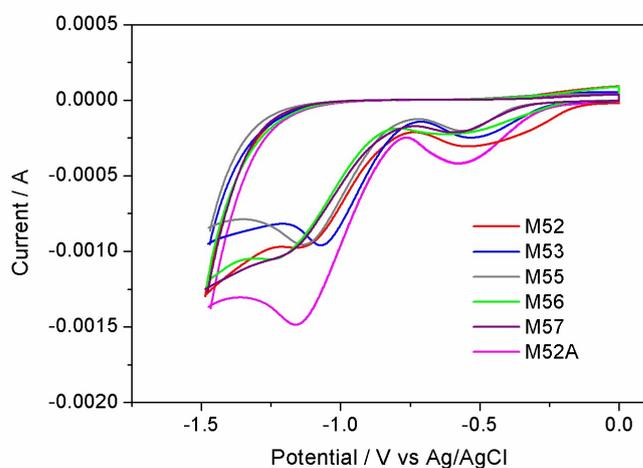
**Fig. S2.** CV of sensitized electrodes between 0 to  $-1.5 \text{ V}$ .
