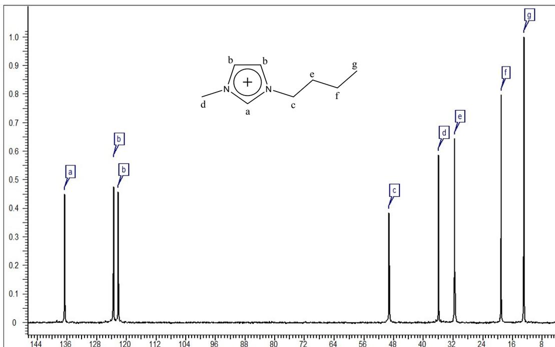
(e)  $^1\text{H}$  NMR spectrum of  $[\text{C}_6\text{C}_1\text{im}][\text{ClO}_4]$  in  $\text{DMSO-D}_6$  as solvent at 200 MHz
