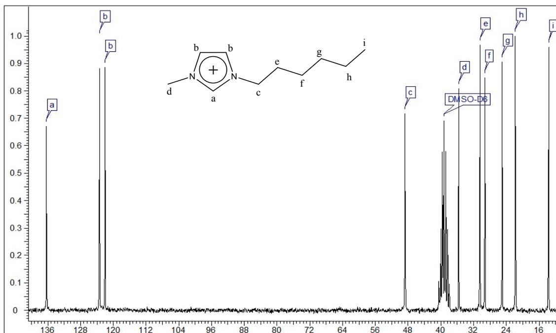
(g)  $^1\text{H}$  NMR spectrum of  $[\text{C}_8\text{C}_1\text{im}][\text{ClO}_4]$  in  $\text{DMSO-D}_6$  as solvent at 200 MHz
