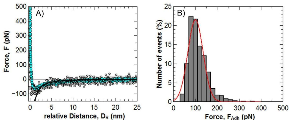
**Figure S2** A) Typical force vs distance profile (approach only, single profile in grey) and mean curve of about 15 approach profiles (blue) measured for the  $L_0/L_0$  setup. B) Adhesion measured for the same setup.
