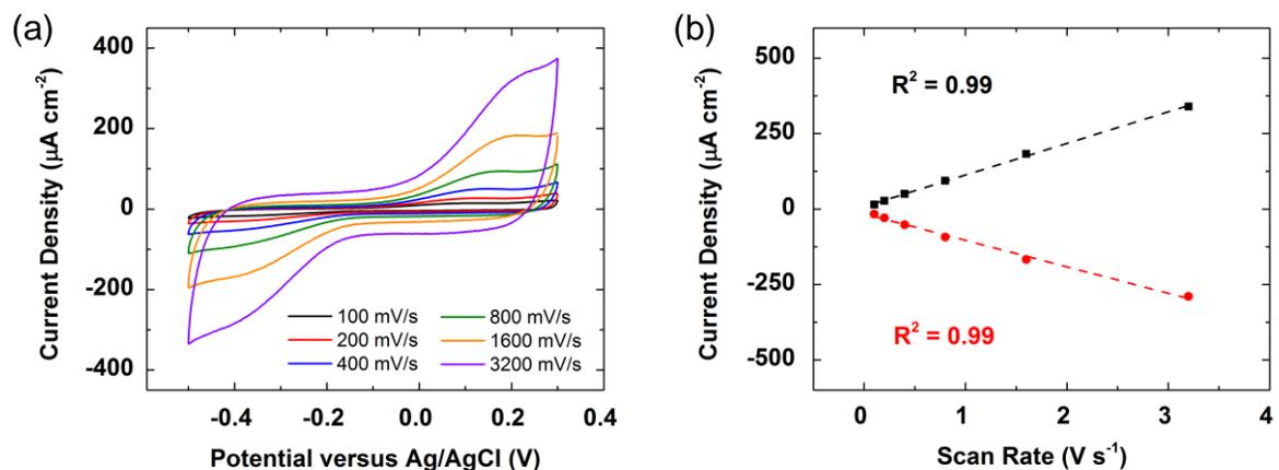
**Figure S4.** (a) CVs of a SAM of BHQ covered by a DMPC monolayer in pH 7 Ar-saturated solution at various scan rates. (b) Randles-Sevcik plot of the peak anodic (black) and cathodic (red) current densities of a SAM of BHQ covered by a DMPC monolayer versus scan rate.
