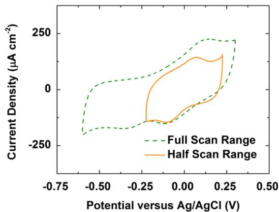
**Figure S11a.** CVs of a SAM of BHQ covered by a monolayer of DMPC with 1 equivalent of MDP added scanning the full range (dashed green) and half range (solid orange) in an Ar-saturated pH 7 solution at a scan rate of 1600 mV/s.
