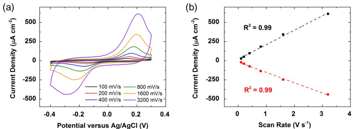
**Figure S1.** (a) CVs of a SAM of BHQ on Au in pH 3 Ar-saturated solution at various scan rates. (b) Randles-Sevcik plot of the peak anodic (black) and cathodic (red) current densities of a SAM of BHQ versus scan rate.
