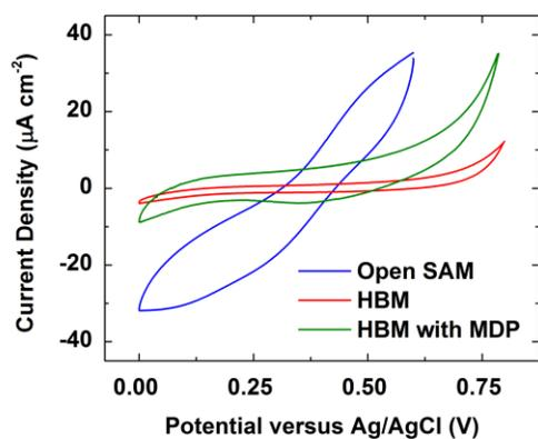
**Figure S15.** CVs of a SAM of  $N_2$ -BHQ (blue), the  $N_2$ -BHQ-containing HBM (red), and the  $N_2$ -BHQ-HBM with MDP incorporated in the lipid layer (green) in a solution of  $K_3Fe(CN)_6$  (1 mM) with KCl (100 mM) at a scan rate of 50 mV/s.
