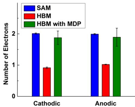
**Figure S9.** Bar graphs showing the number of electrons transferred for the cathodic and anodic processes of a SAM of BHQ (blue) covered by a monolayer of DMPC (red) with 1 equivalent of MDP incorporated in the lipid layer (green) in pH 5 Ar-saturated solution.
