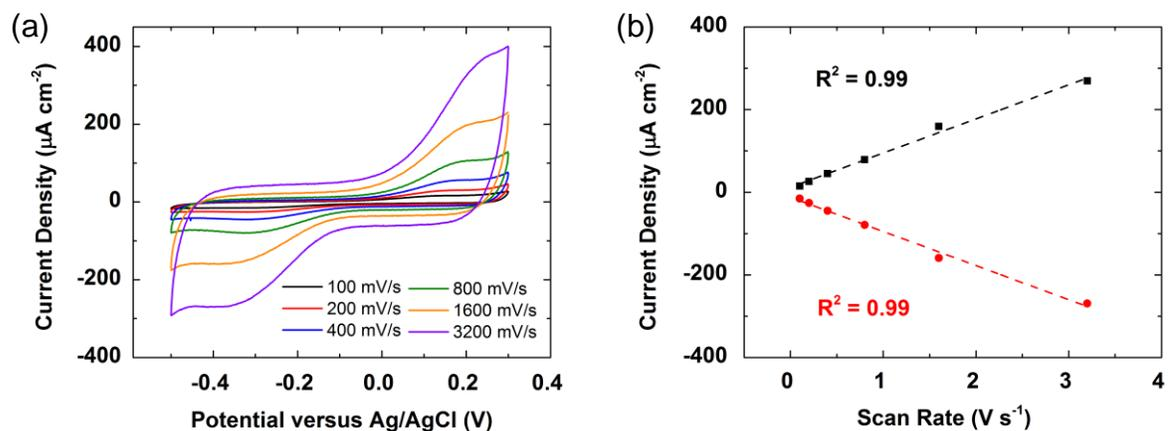
**Figure S5.** (a) CVs of a SAM of BHQ covered by a DMPC monolayer in pH 5 Ar-saturated solution at various scan rates. (b) Randles-Sevcik plot of the peak anodic (black) and cathodic (red) current densities of a SAM of BHQ covered by a DMPC monolayer versus scan rate.
