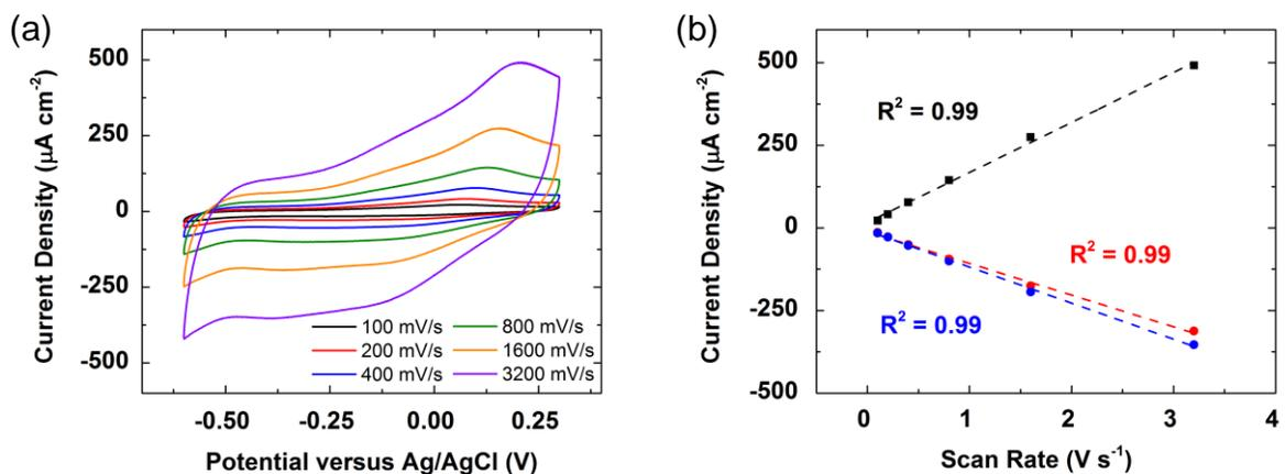
**Figure S7.** (a) CVs of a SAM of BHQ covered by a DMPC monolayer with 1 equivalent of MDP incorporated in the lipid layer in pH 5 Ar-saturated solution at various scan rates. (b) Randles-Sevcik plot of the peak anodic (black) and cathodic (red, blue) current densities of a SAM of BHQ covered by a DMPC monolayer with MDP incorporated in the lipid layer versus scan rate.
