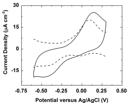
**Figure S11b.** CV of a SAM of BHQ covered by a monolayer of DMPC with 0.2 equivalents of MDP added in an Ar-saturated pH 7 solution at a scan rate of 100 mV/s (solid line). Square wave voltammetry of the same system performed using an increment voltage of 4 mV, an amplitude of 25 mV, and a frequency of 15 Hz.
