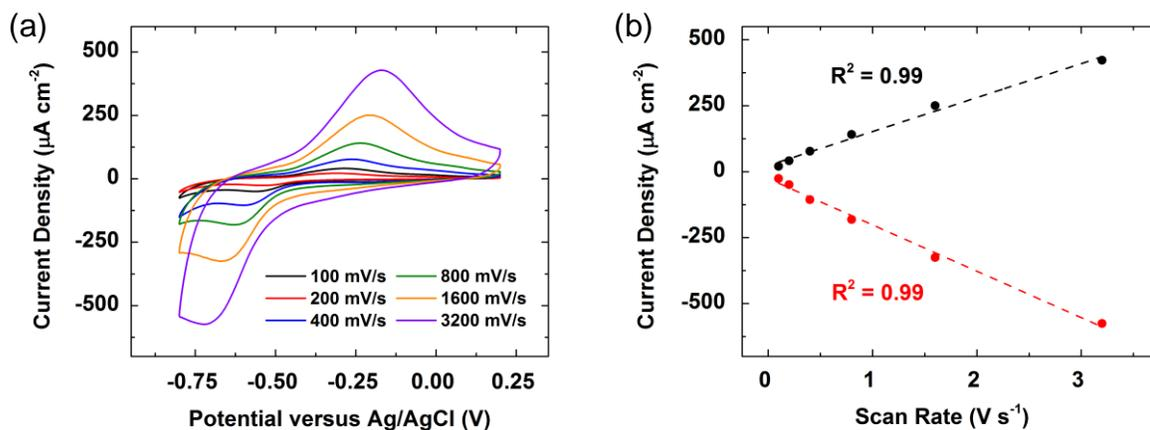
**Figure S13.** (a) CVs of a SAM of N<sub>2</sub>-BHQ on Au in pH 7 Ar-saturated solution at scan rates of 100 (black), 200 (red), 400 (blue), 800 (green), 1600 (orange), and 3200 (purple) mV/s. (b) Randles-Sevcik plot of the peak anodic (black) and cathodic (red) current densities of a SAM of N<sub>2</sub>-BHQ versus scan rate.
