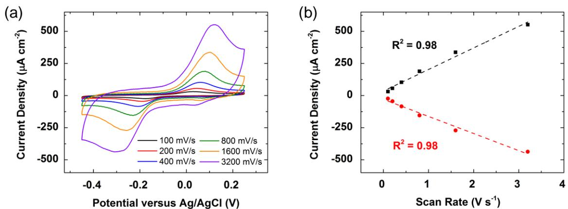
**Figure S2.** (a) CVs of a SAM of BHQ on Au in pH 5 Ar-saturated solution at various scan rates. (b) Randles-Sevcik plot of the peak anodic (black) and cathodic (red) current densities of a SAM of BHQ versus scan rate.
