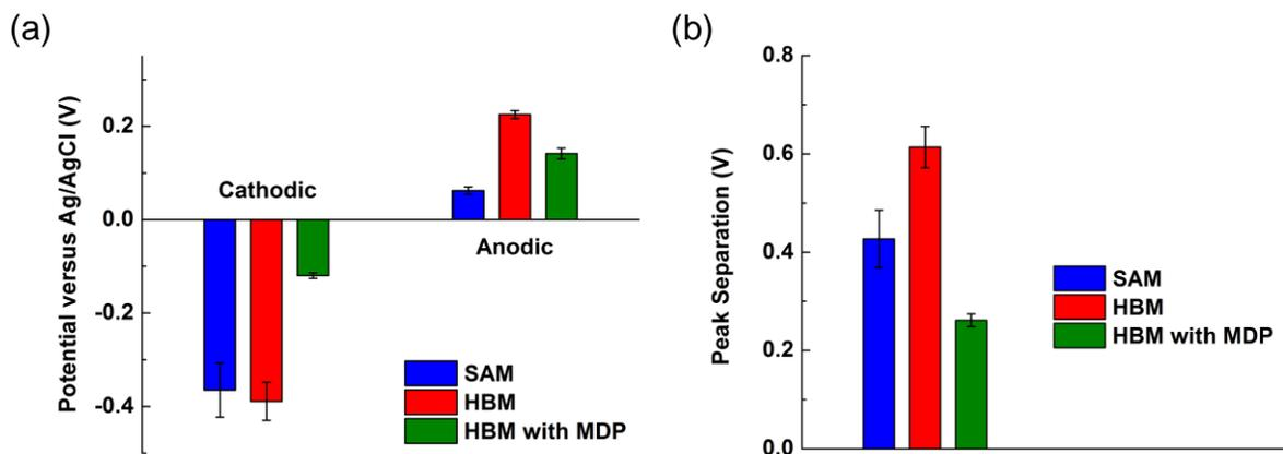
**Figure S8.** Bar graphs showing BHQ (a) cathodic and anodic peak positions and (b) peak separations at pH 7. Each graph has three sets of bars: open SAM, HBM, and HBM with 1 equivalent of MDP. For HBM with MDP, the cathodic peak position of the more negative cathodic wave is  $-0.374 \pm 0.022$  V versus Ag/AgCl.
