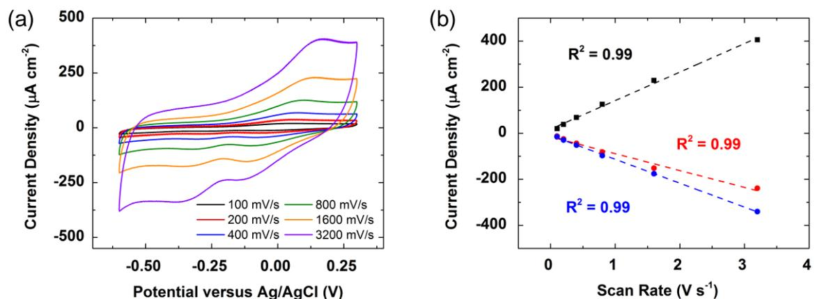
**Figure S6.** (a) CVs of a SAM of BHQ covered by a DMPC monolayer with 1 equivalent of MDP incorporated in the lipid layer in pH 7 Ar-saturated solution at various scan rates. (b) Randles-Sevcik plot of the peak anodic (black) and cathodic (red, blue) current densities of a SAM of BHQ covered by a DMPC monolayer with MDP incorporated in the lipid layer versus scan rate.
