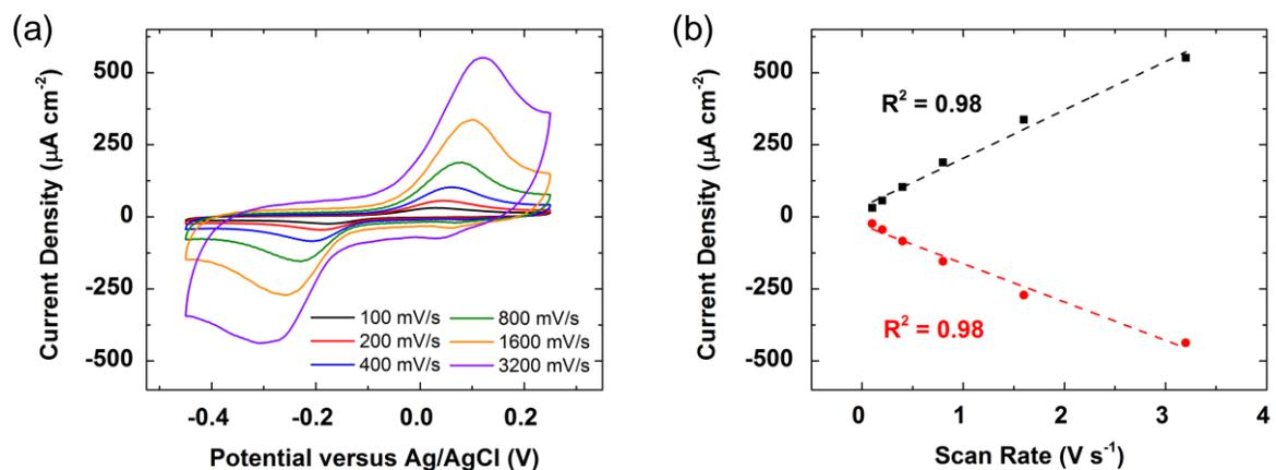
**Figure S3.** (a) CVs of a SAM of BHQ on Au in pH 9 Ar-saturated solution at various scan rates. (b) Randles-Sevcik plot of the peak anodic (black) and cathodic (red) current densities of a SAM of BHQ versus scan rate.
