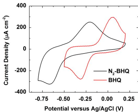
**Figure S12.** CVs of a SAM of BHQ (red) and a SAM of N<sub>2</sub>-BHQ (black) on Au in pH 7 Ar-saturated solution at scan rates of 1600 mV/s.
