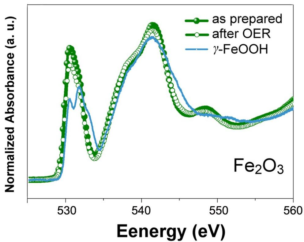
**Figure S2.** XANES spectra of O *K*-edge for  $\gamma$ -Fe<sub>2</sub>O<sub>3</sub>.
