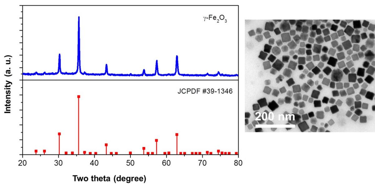
**Figure S1.** XRD spectrum and corresponding TEM image of  $\gamma$ - $\text{Fe}_2\text{O}_3$  reference sample.
