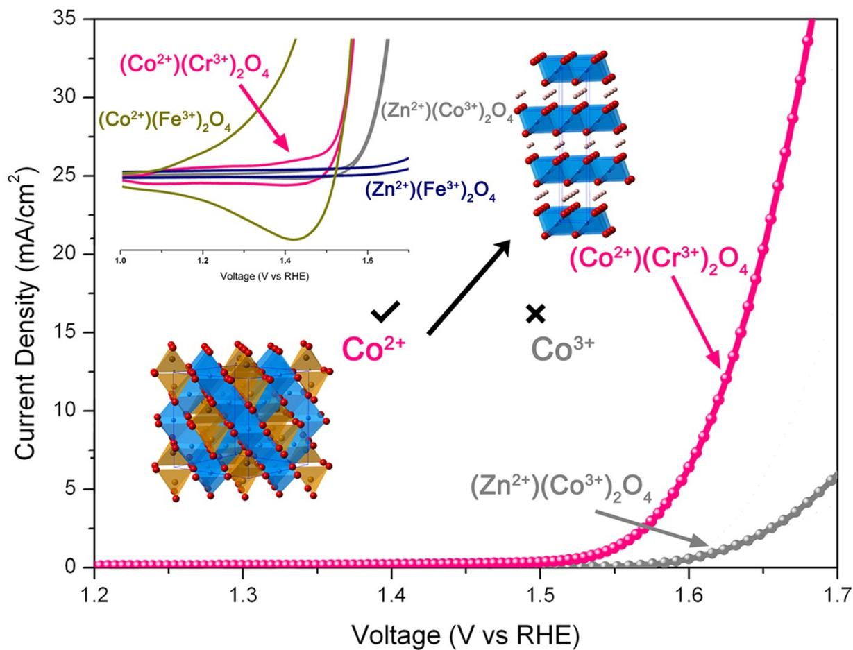
**Figure S4.** Electrochemical performance for ZnCo<sub>2</sub>O<sub>4</sub> and CoCr<sub>2</sub>O<sub>4</sub>, the OER polarization curves were performed upon a GC-RDE system in alkaline electrolyte (0.5M KOH; pH~13.6). Insert: Cyclic voltammogram of ZnCo<sub>2</sub>O<sub>4</sub>, CoCr<sub>2</sub>O<sub>4</sub>, ZnFe<sub>2</sub>O<sub>4</sub>, and CoFe<sub>2</sub>O<sub>4</sub>.
