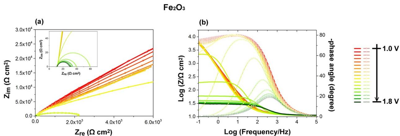
**Figure S8.** Electrochemical impedance spectra of Fe<sub>2</sub>O<sub>3</sub> present Nyquist (a) and Bode (b) plots.
