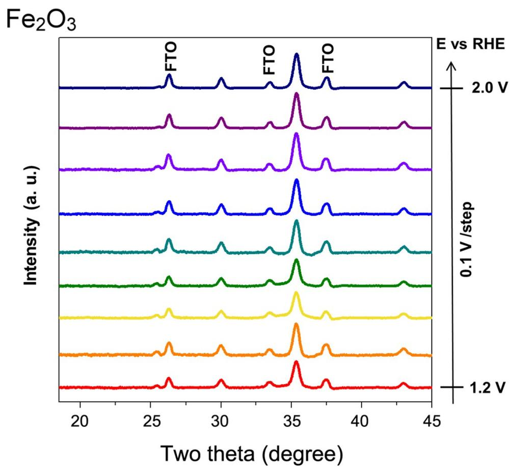
**Figure S3.** *In-situ* XRD spectra of  $\gamma\text{-Fe}_2\text{O}_3$  sample, an electrolyte of 0.5 M KOH was employed with a potential range from 1.2 to 2.0 V vs RHE.
