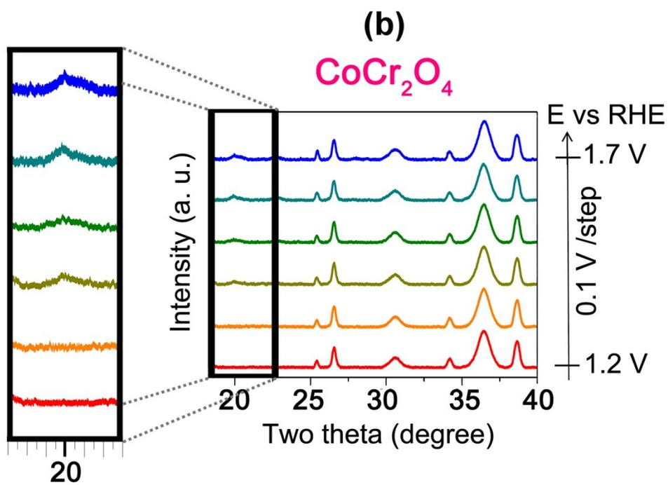
**Figure S5.** *In-situ* XRD spectra of  $\text{ZnCo}_2\text{O}_4$  and  $\text{CoCr}_2\text{O}_4$  samples, a KOH electrolyte of 0.5 M was employed and all measurements with a potential range from 1.2 to 1.7 V vs RHE were operated potentiostatically.
