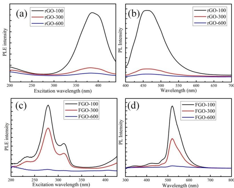
Figure S2. PLE spectrum from rGOs (rGO-100, rGO-300 and rGO-600) (a). PL spectrum from rGOs with the detection wavelength of 386nm (b). And PLE spectrum (c) and PL spectrum with
