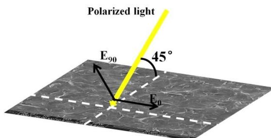
Figure S1. The scheme of polarized ATR-FTIR.
