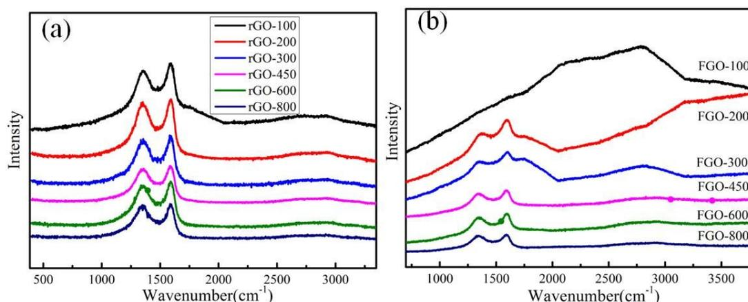
Figure S3. The Raman spectrum of rGOs thermal reduction at different temperatures and their corresponding FGOs.
