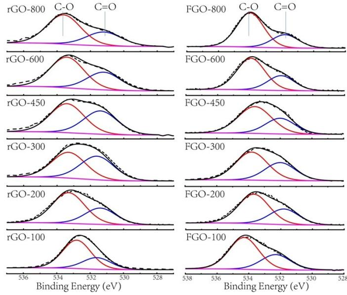
Figure S6. XPS O 1<sub>s</sub> spectra of GOs with different thermal reduction temperature and their corresponding FGOs.
