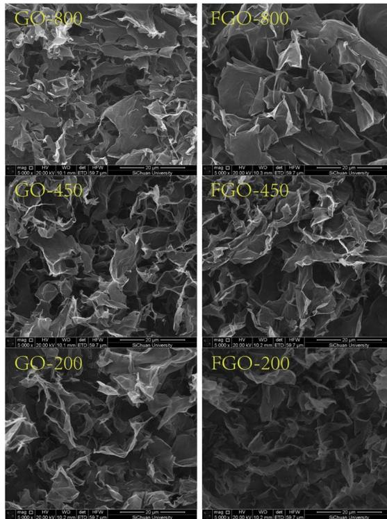
Figure S4. SEM micrographs of sample rGO-800, rGO-450, rGO-200 and their corresponding fluorinated products, FGO-800, FGO-450, FGO-200.
