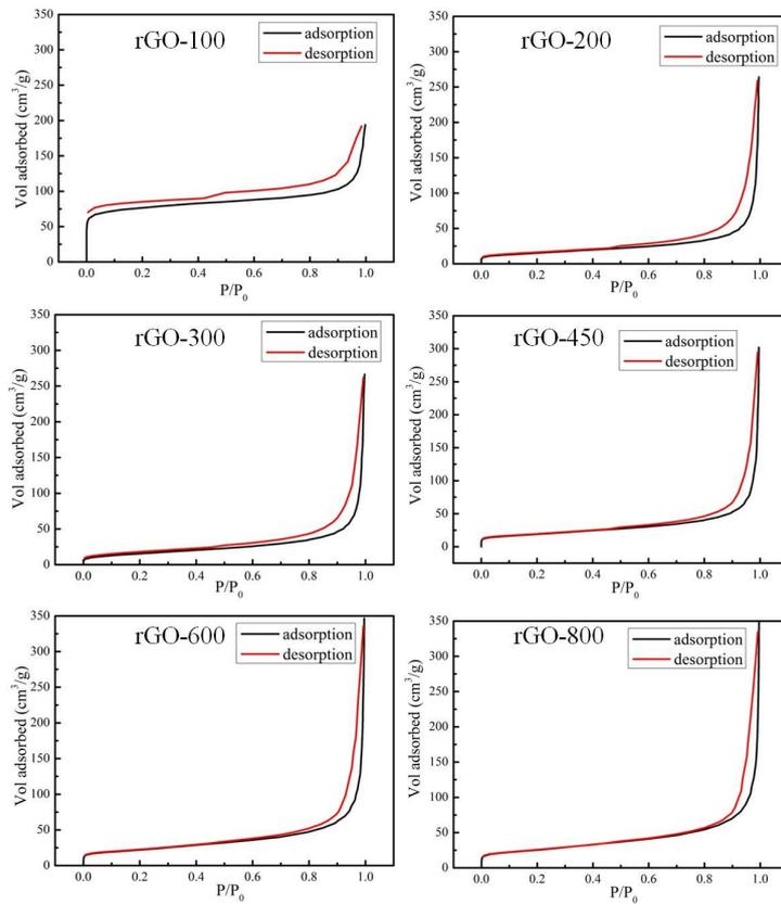
Figure S5. Nitrogen sorption isotherms of rGOs with different oxygen contents.
