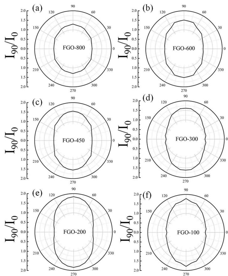
Figure S7. Polar diagrams of absorbance of peaks at  $1140\text{cm}^{-1}$  for FGOs.
