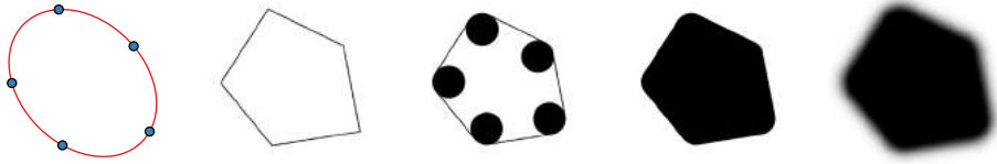
FIG. S3: Construction of a polygon on a discrete grid, having rounded corners and a fuzzy boundary. (a, b) The corner points are defined by polar coordinates with respect to the center of the ellipse. (c) The inscribed circle is drawn at every corner. (d) The interior is filled using a hole-filling algorithm. (e) The edges are drawn with a Gaussian intensity profile.
