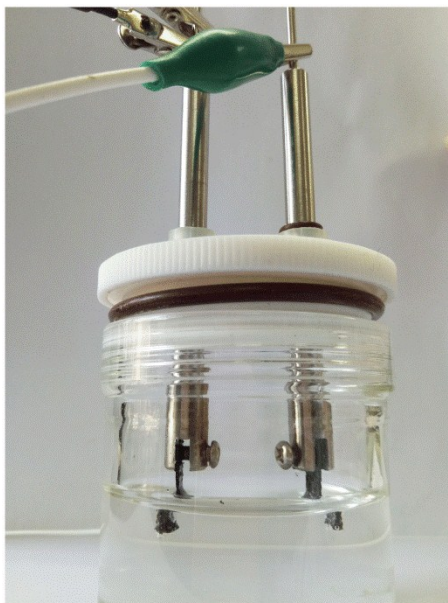
Fig. S6 Photograph showing the generation of hydrogen and oxygen bubbles from overall water splitting on \text{CoS}_2/\text{GF} electrodes in a two-electrode configuration.
