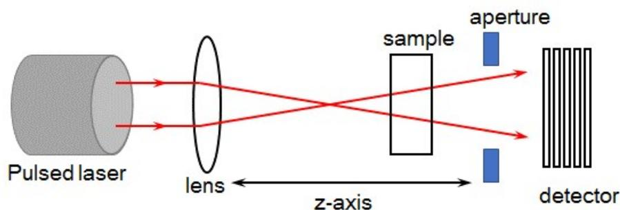
**Fig. s2.** Illustration of the experiment set for Z-scan.
