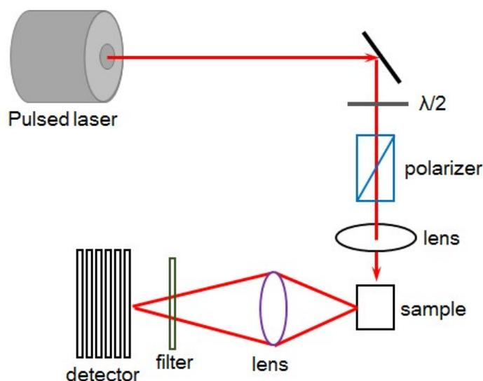
**Fig. s1.** Illustration of experiment set for two-photon excited fluorescence (TPEF) technique.
