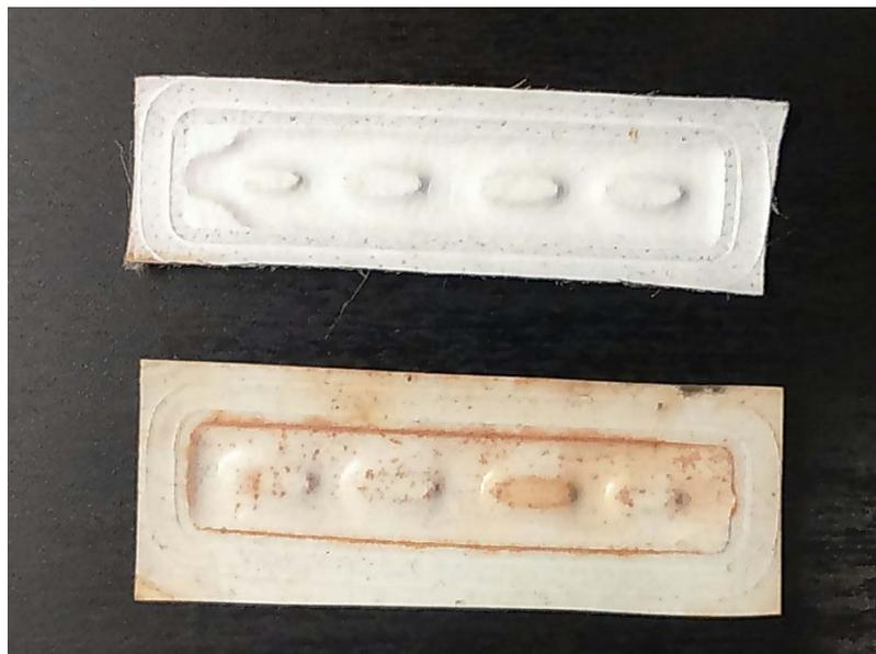
**Figure S6.** Visual inspection of the size-exclusion membrane; (up) pristine size-exclusion membrane; (down) size-exclusion membrane after a single Appel reaction run using 1-nonanol as substrate. The dendrimer catalyst has been partially retained on the membrane surface, possible due to the low solubility of the macromolecular catalyst in the organic solvents employed.
