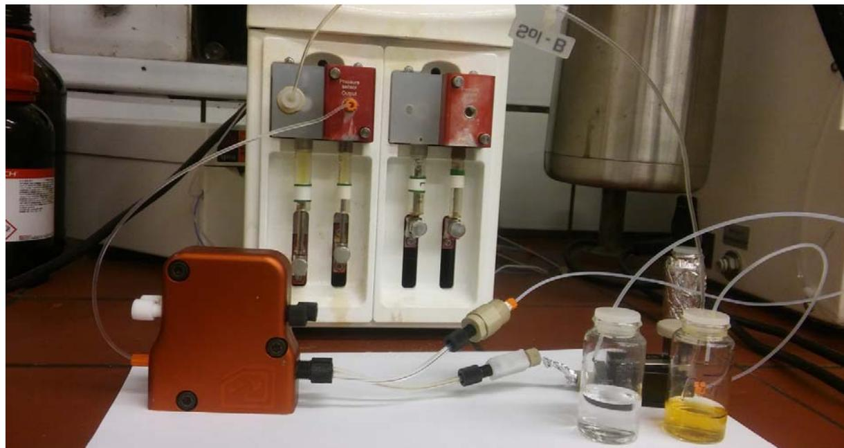
**Figure S2.** The purification of the bypyridine-dendrimer was done through nanofiltration in methanol with the size-exclusion membrane (NF080105, Solsep BV, The Netherlands) installed in a commercial liquid-liquid separator system (Zaiput). Left vial: filtered solution; right vial: retentate solution. The concentration of the dendrimer was 30 mg/mL (400 mg in 15 mL). The filtration was performed at 12.5 bar and a flow rate of 0.2 mL/min. We obtained 58% of the volume in the filtrate.
