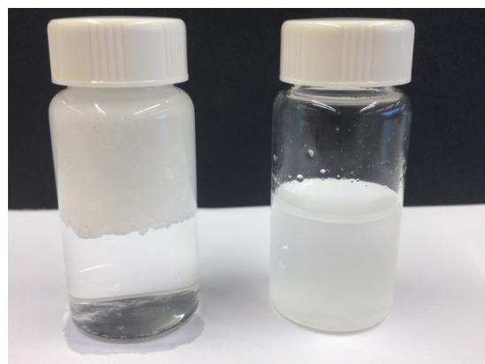
**Figure S5-** m-MCF-60 functionalized with n-propyl groups (left) and pristine m-MCF-60 (right) mixed with water.
