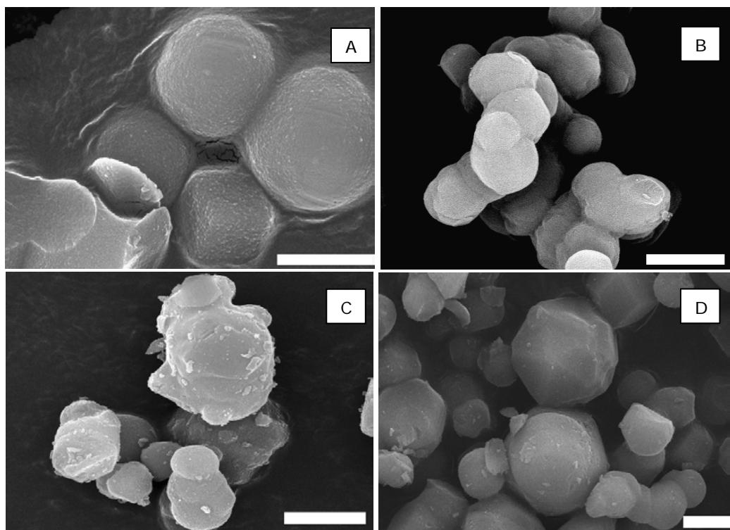
**Figure S4-** SEM images pristine materials (A) SBA16-A-373-5.5 (B) SBA16-A-373-24 (C)SBA16-B-353-24 (D)SBA16-C-373-24, scale bars:2 $\mu$ m
