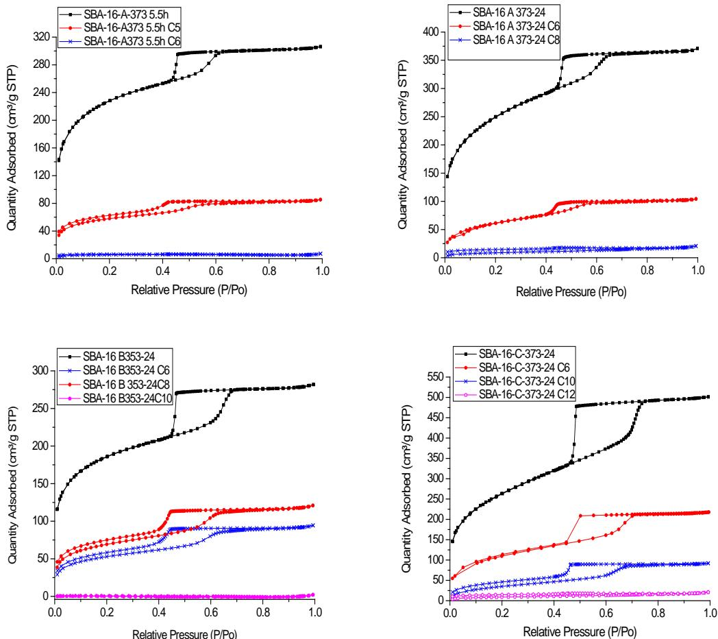
**Figure S1- Nitrogen adsorption isotherms to determine the window size of SBA-16 materials after functionalization**
