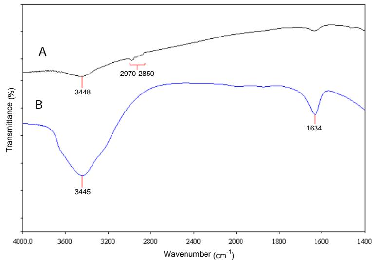
**Figure S7-IR spectra (A) Functionalized MCF-60 with n-propyl groups (B) pristine m-MCF-60**
