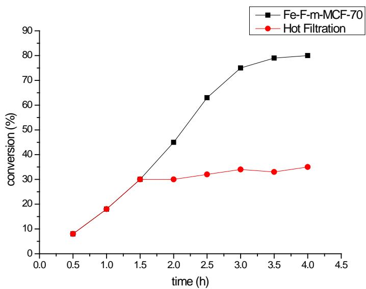
**Figure S12- Time-conversion plot and leaching test as evidence for the nature of the catalyst for sulfoxidation of benzyl phenyl sulfide**
