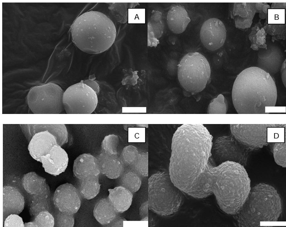
**Figure S3- SEM images of pristine materials (A) m-MCF-50, (B)m-MCF-60, (C)m-MCF-70 and (D) m-MCF-80 Scale Bars: 2µm**
