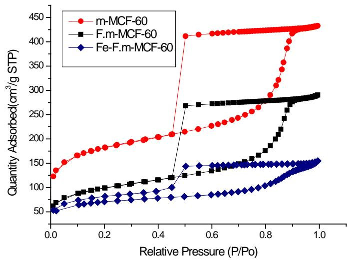
Figure S9-N<sub>2</sub> Physisorption at 77K of m-MCF-60, F.m-MCF-60 and Fe.F.m-MCF-60
