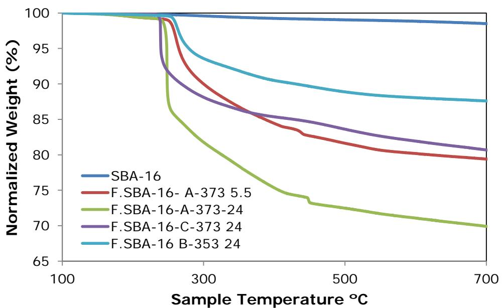
**Figure S8-** TGA analysis of a pristine m-MCF and functionalized m-MCFs (top frame) and a pristine SBA-16 and functionalized SBA-16 (bottom frame)
