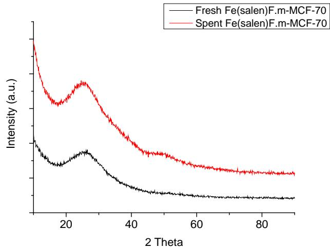
Figure S10- XRD analysis of fresh and spent Fe(salen) F.m-MCF-70
