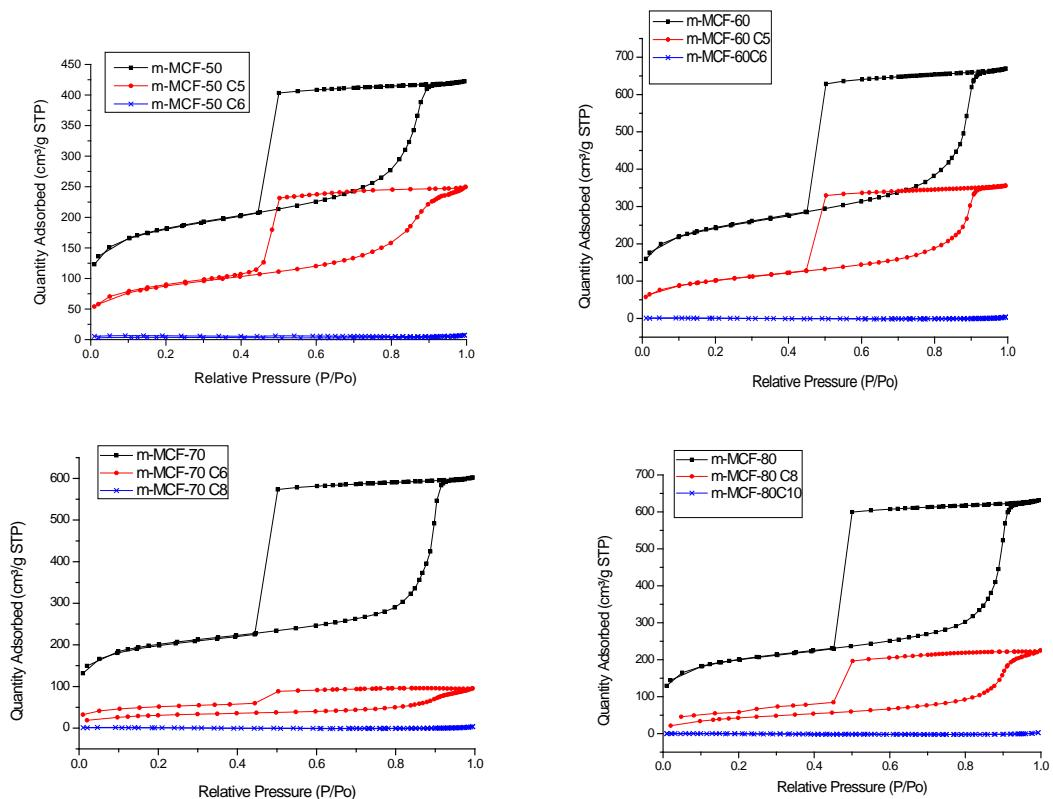
**Figure S2- Nitrogen adsorption isotherms to determine the window size of m-MCF materials after functionalization**
