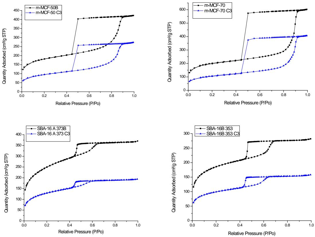
**Figure S6- N<sub>2</sub> physisorption of pristine material and the respective material functionalized with n-propyl groups**
