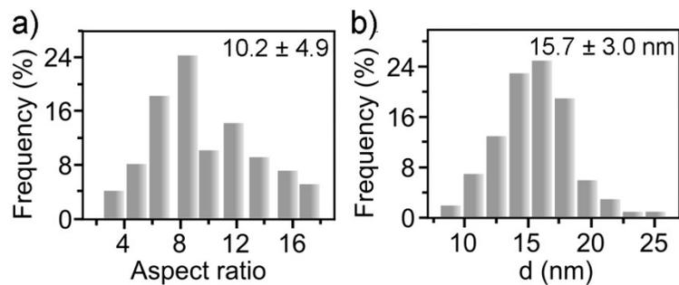
**Fig. S1** a) Distributions of aspect ratio calculated for the as-prepared nanoparticle-decorated CdS microrods, and b) the diameter calculated for the surface nanoparticles. All the calculations were performed by measuring 100 rods/particles shown in a low-resolution SEM image ( $n = 100$ ).
