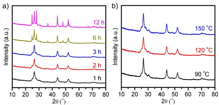
**Fig. S2** XRD patterns of CdS samples synthesized using a standard process except that a) different reaction times, and b) different reaction temperatures were employed.
