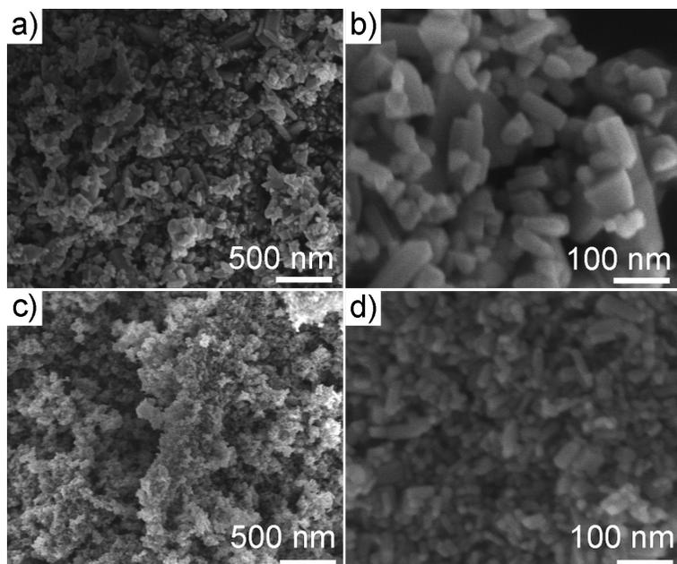
**Fig. S5** SEM images of CdS samples synthesized using a standard process except that the reactions were proceeded in the absence of a, b) EN, and c, d) NaOH. b) and d) are corresponding magnified images.
