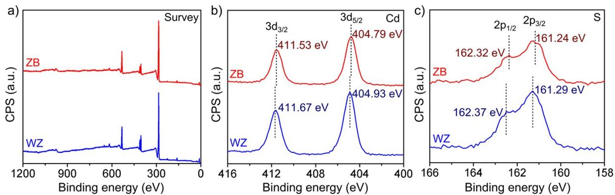
**Fig. S8** XPS spectra of ZB CdS nanoparticles (obtained using a standard synthesis except the temperature was set to 150 °C) and WZ CdS microrods (obtained in pure EN). a) survey spectra, and b, c) the corresponding high-resolution elemental scans of Cd 3d, and S 2p, respectively.
