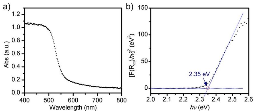
**Fig. S4** (a) UV-vis spectra of the as-prepared CdS photocatalyst using a standard synthesis except the temperature was set to 150 °C, and (b) the corresponding K-M plot showing its band-gap energy.
