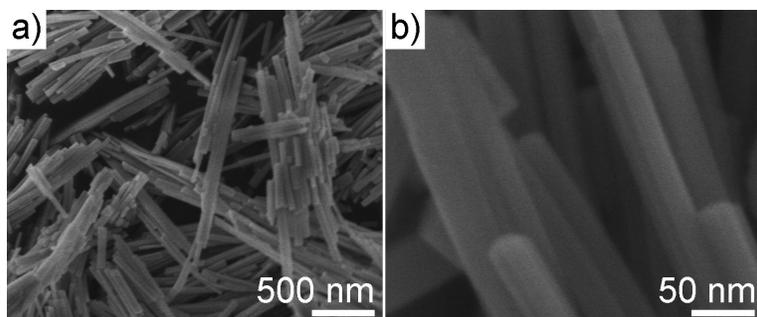
**Fig. S7** The SEM images of CdS microrods synthesized in pure EN solution.
