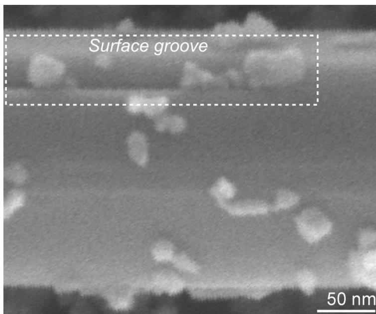
**Fig. S6** Magnified SEM images of a single CdS microrod synthesized using a standard process except the reaction was allowed for 18 h. The image shows a clear surface groove structure for the following regrowth of CdS monomers.
