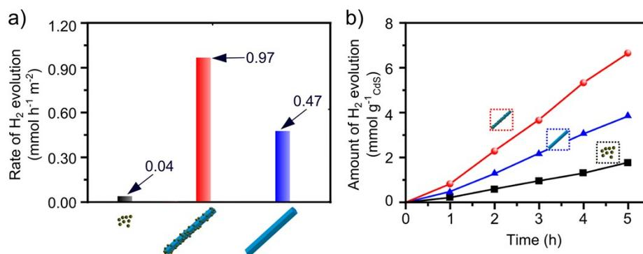
**Fig. S9** Visible-light-driven H<sub>2</sub> evolution from an aqueous solution containing 0.35 M of Na<sub>2</sub>S, 0.25 M of Na<sub>2</sub>SO<sub>3</sub>, and 100 mg of CdS photocatalyst. a) Specific activities of the as-prepared CdS nanoparticles, nanoparticle-decorated microrods, and pure microrods, by normalizing the initial average hydrogen evolution rates with respect to their BET specific areas, and b) the corresponding time courses of photocatalytic hydrogen production.
