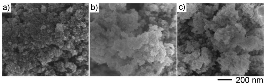
**Fig. S3** SEM images of CdS photocatalysts synthesized using a standard process except that the reaction temperatures were tuned to a) 90 °C, b) 120 °C, and c) 150 °C, respectively.
