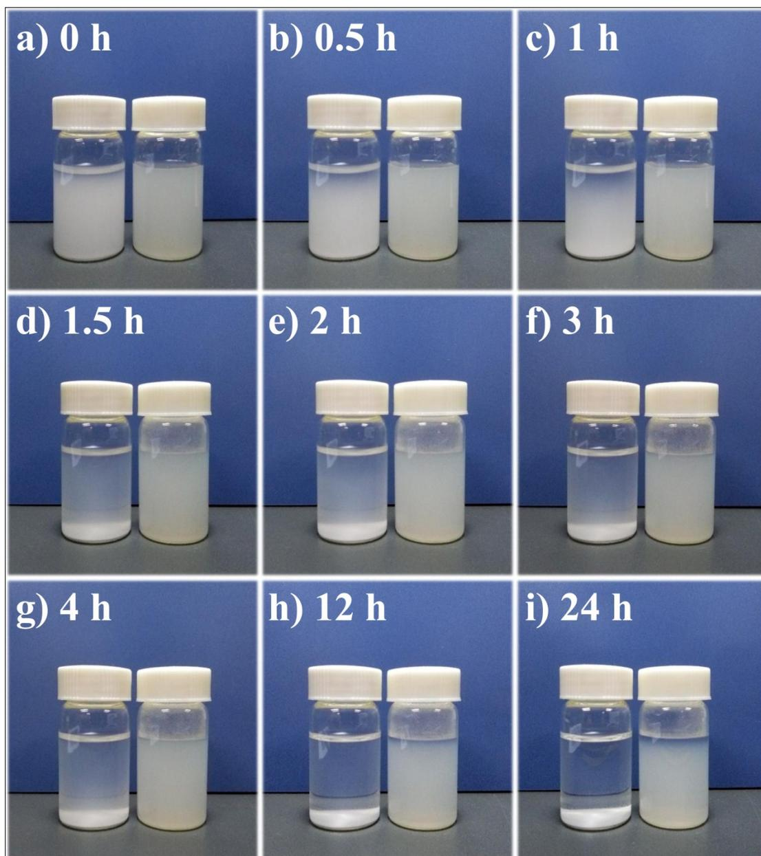
**Fig. S3** Images of anatase sphere (left) and TiO<sub>2</sub>@h-CeO<sub>2</sub> (right) suspensions kept steady for different times. The contents of both materials were 1 mg/ mL. And the suspensions were treated with ultrasonication for 30 min before kept steady.
