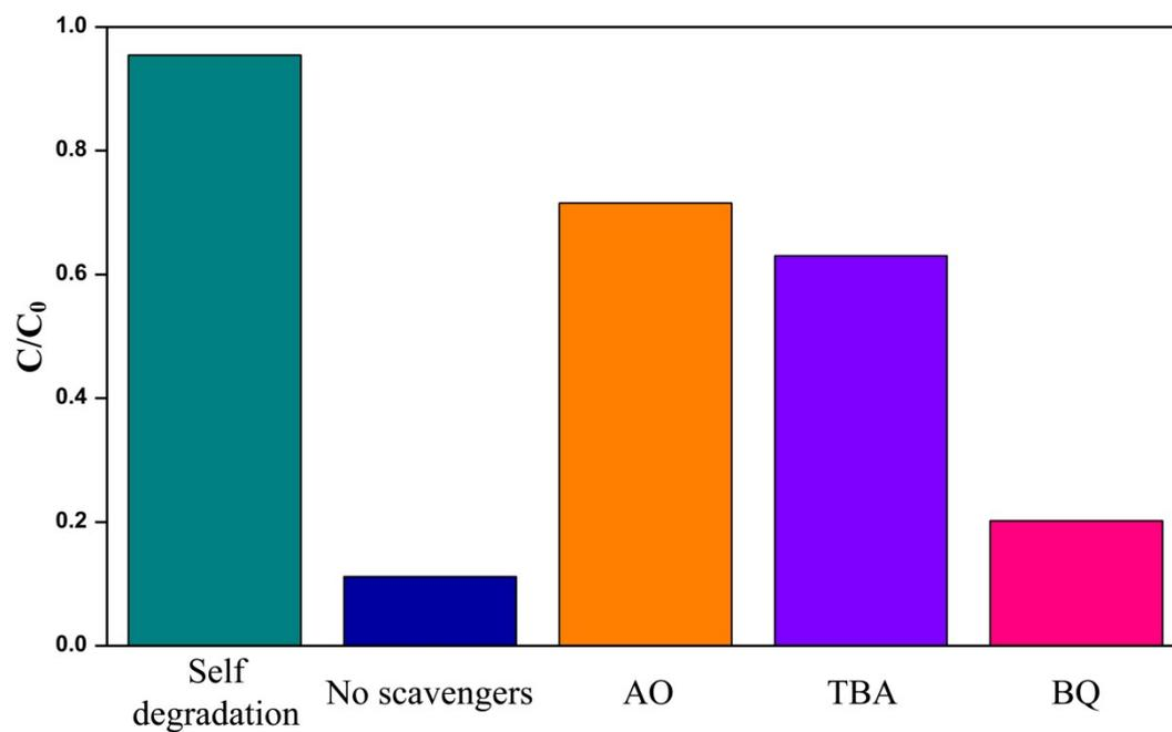
**Fig. S5** Trapping experiment of active species during the photocatalytic degradation with 20 min high-pressure mercury lamp irradiation.
