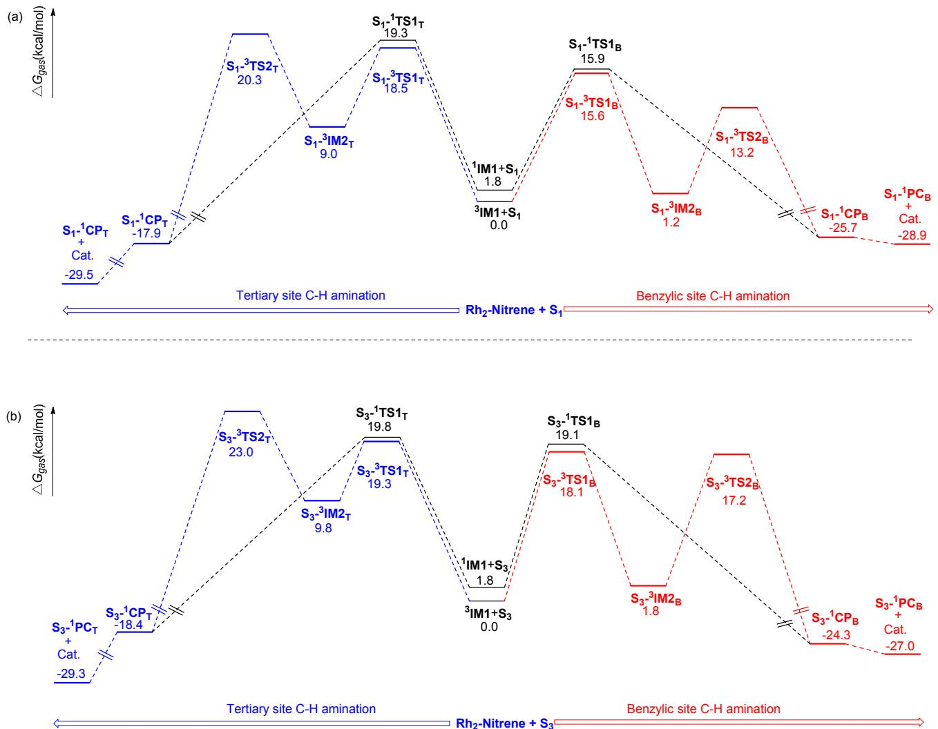
**Fig. S5 (a) (b)** Free energy profiles of intermolecular C-H aminations for the isoamylbenzene-derived substrate **S<sub>1</sub>** and **S<sub>3</sub>**, respectively.
