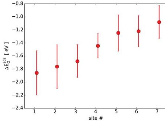
Figure S9: Adsorption energy of oxygen on different sites on the lowest-energy cluster. More negative means stronger binding.
