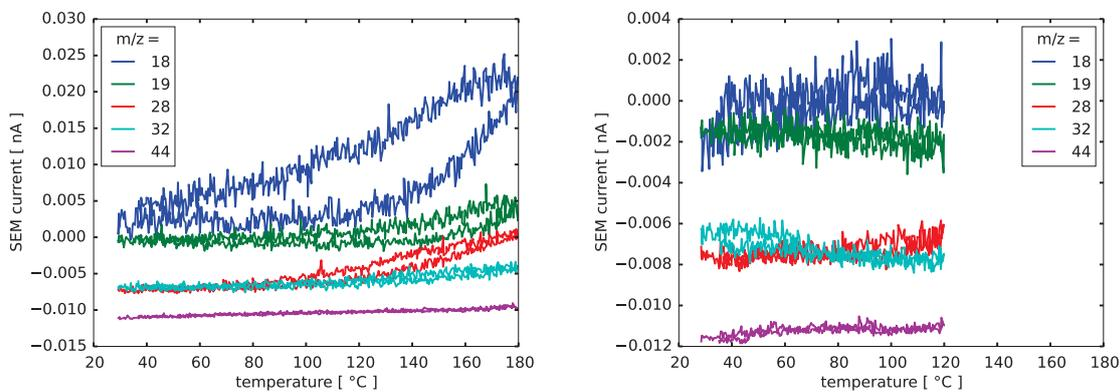
Figure S7: Signals from bi-products measured during HD production of the  $\text{Pt}_8$  sample. Left shows signals during pure  $\text{H}_2/\text{D}_2$  dosage and right show the same signals while dosing 26 ppm  $\text{O}_2$ .
