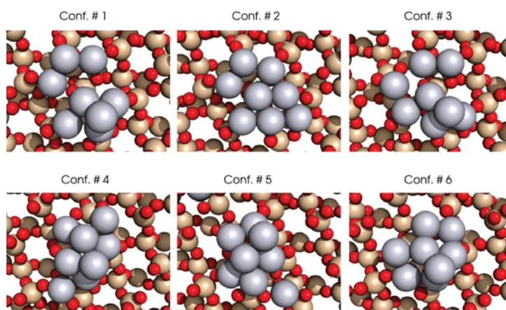
Figure S8: Relaxed atomic configurations ordered by decreasing binding energy. Atoms are color coded; platinum (grey), silicon (golden), and oxygen (red).
