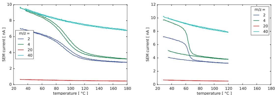
Figure S6: Reactant signals measured during HD production of the  $\text{Pt}_8$  sample. Left shows signals during pure  $\text{H}_2/\text{D}_2$  dosage and right show the same signals while dosing 26 ppm  $\text{O}_2$ .
