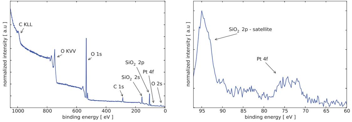
Figure S4: XPS spectra of the  $\text{Pt}_8$  sample after chemical testing. Left shows an overview scan. Right shows a zoom in on the  $\text{SiO}_2$  satellite peak and the Pt doublet peak.
