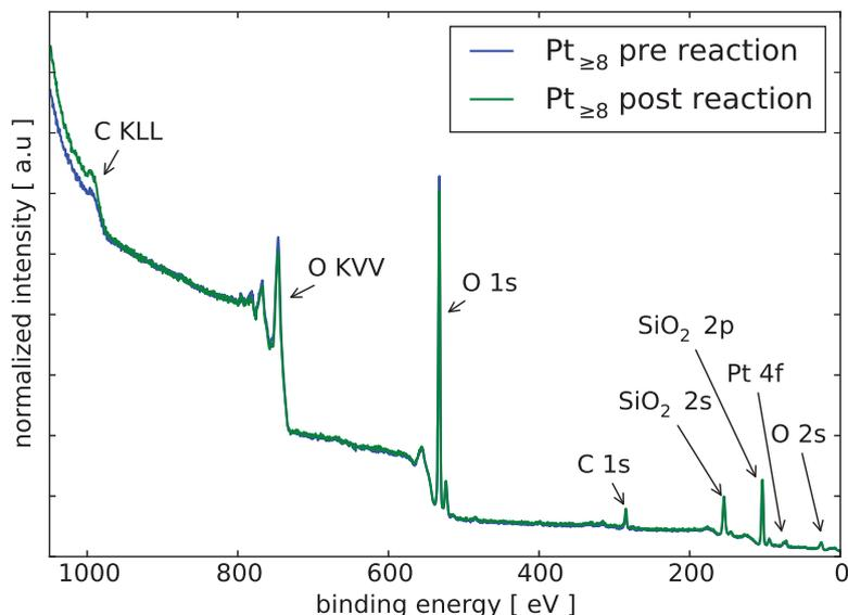
Figure S3: XPS overview spectra of  $\text{Pt}_{\geq 8}$  before (blue) and after (green) chemical activity testing.
