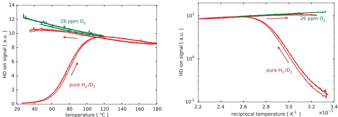
Figure S5: Left shows the HD production as function of temperature from the  $\text{Pt}_{\geq 8}$  sample. An Arrhenius plot of the same data is shown on the right.
