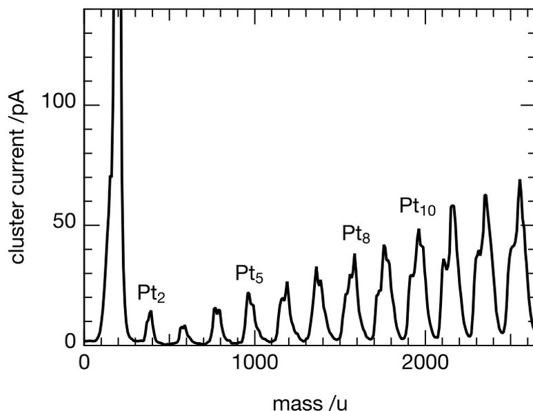
Figure S1: Mass scan of the cluster current. A clear separation of the cluster peaks indicates mono-disperse clusters during deposition.
