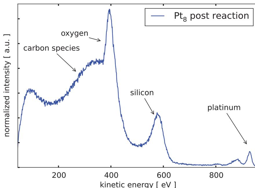
Figure S2: ISS spectra of  $\text{Pt}_8$  after chemical activity testing.
