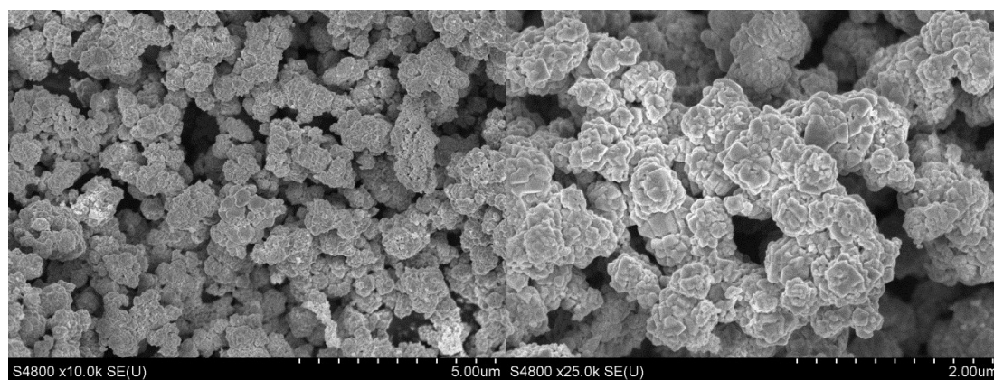
Fig. S7 FE-SEM patterns of [PYD]@Cu (up) with different magnification, left (10k), right (25k);
