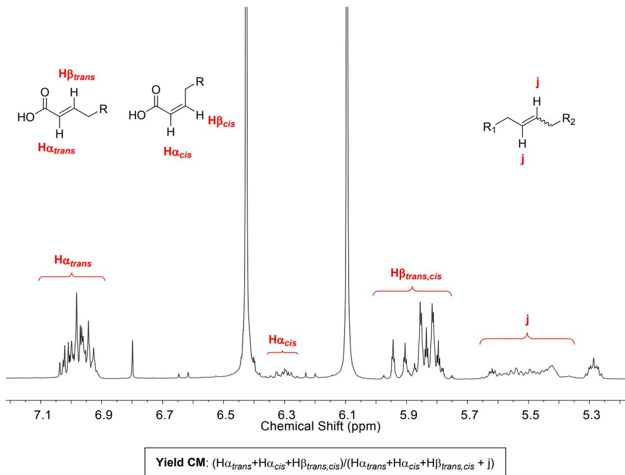
**Figure S4** Inset of the olefinic region of a typical  $^1\text{H}$  NMR spectrum of the CM of vegetable oils with **MA-H** with the signal attributions and the formula used to calculate the yield of cross-metathesis products.
