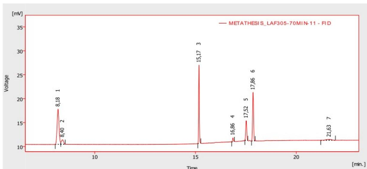
**Figure S2** Typical chromatogram obtained in the cross-metathesis of **MO** with **MA-H** (after derivatization). Methyl 2-undecenoate (8.18 min); 9-octadecene (8.40 min); internal standard (1,3,5-trimethoxybenzene; 15.17 min); unknown compound (16.86 min); methyl oleate (17.52 min); dimethyl 2-undecenedioate (17.86 min); dimethyl 9-octadecenedioate (21.63 min).
