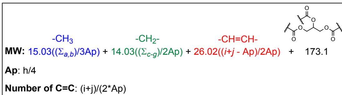
**Figure S3** Typical <sup>1</sup>H NMR spectrum of a vegetable oil with the signal attributions and the formulae used to calculate the molecular weight and number of C-C double bonds per triglyceride. \* Residual water.
