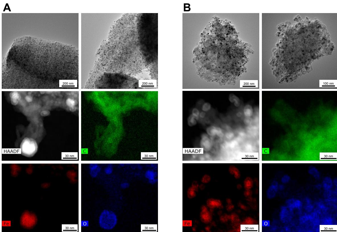
**Fig. S5.** TEM images and EDX elemental mapping TEM images of the spent Fe@CMK-3-500 catalyst (FTO at 1 bar) after (A) activation at 350°C (after 20 h TOS) and (B) activation at 450°C (after 17 h TOS). (Iron-red; Oxygen-blue; Carbon-green).
