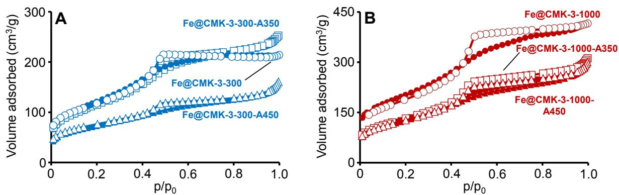
**Fig. S6.** Nitrogen adsorption/desorption (filled symbols/empty symbols) isotherms (-196°C) of (A) the Fe@CMK-3-300 catalyst and (B) the Fe@CMK-3-1000 catalyst after calcination (circles), after FTO (at 1 bar) with activation at 350°C (squares, TOS = 20 h) or 450°C (triangles, TOS = 17 h).
