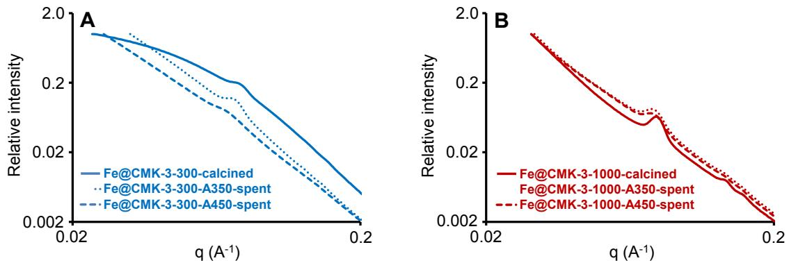
**Fig. S7.** Logarithmic plots of the small-angle X-ray scattering curves of (A) the Fe@CMK-3-300 catalyst and (B) the Fe@CMK-3-1000 catalyst after calcination (straight lines), after FTO (at 1 bar) with activation at 350°C (dotted lines, TOS = 20 h), or 450°C (dashed lines, TOS = 17 h).
