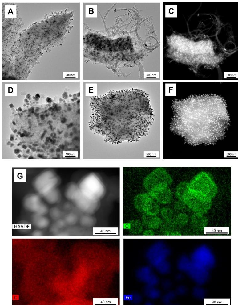
**Fig. S9.** TEM images of the (A-C) Fe@CMK-3-300 and (D-F) Fe@CMK-3-500 catalyst as well as (G) EDX elemental mapping TEM images of Fe@CMK-3-500 after 140 h TOS at GHSV = 9600 h<sup>-1</sup>, H<sub>2</sub>/CO = 2, T = 340°C, p = 10 bar. (Iron-blue; Oxygen-green; Carbon-red).
