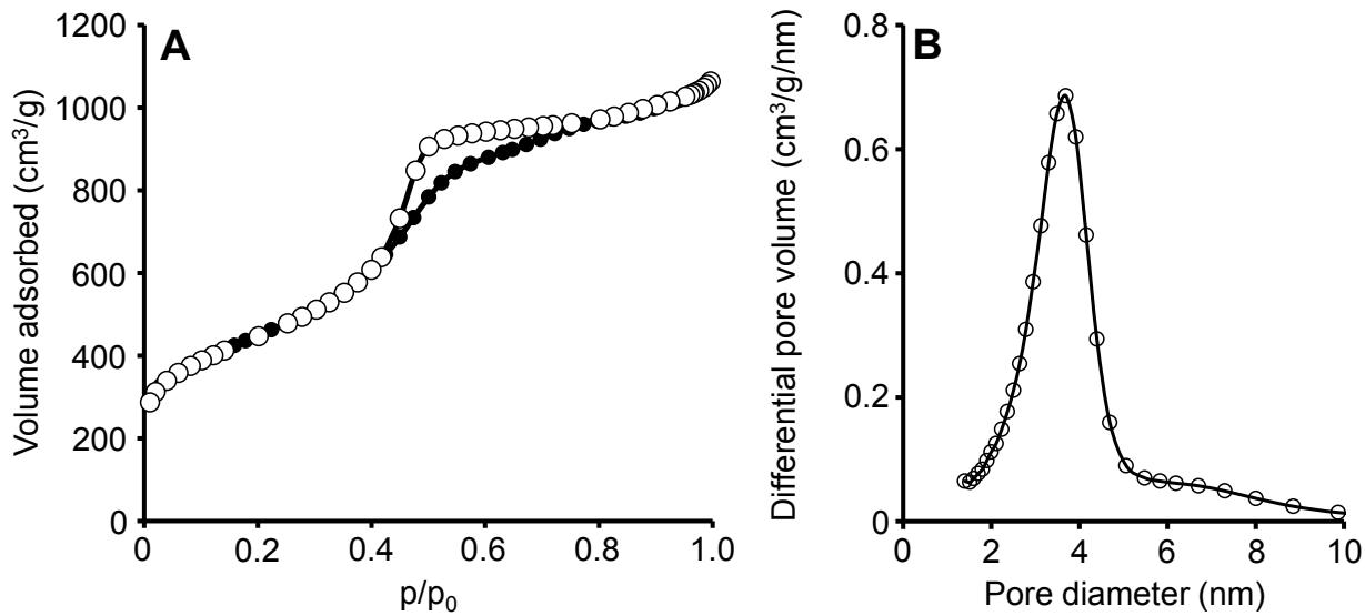
**Fig. S1.** (A) Nitrogen adsorption/desorption (filled symbols/empty symbols) isotherm (-196°C) as well as (B) BJH pore size distribution calculated from the adsorption branch of the pristine CMK-3 support.
