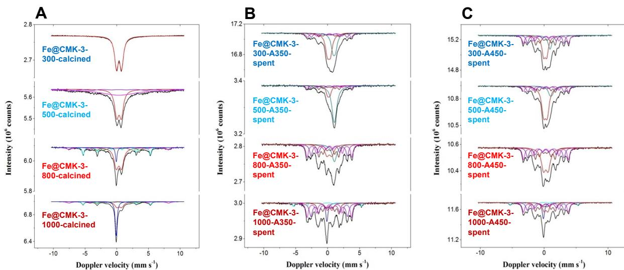
**Fig. S2.** Mössbauer spectra of (A) the catalysts after calcination and the spent catalysts (FTO at 1 bar for 18 h of TOS) after (B) activation at 350°C and (C) activation at 450°C. The assignment of the fitting curves to different iron species can be found in Table S1.
