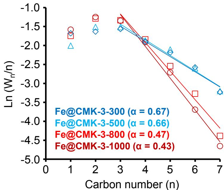
**Fig. S8.** ASF plots of the C<sub>1</sub>-C<sub>7</sub> product fractions as well as chain growth probability ( $\alpha$ ) based on the C<sub>3</sub>-C<sub>7</sub> products of the sodium/sulfur promoted Fe@CMK-3 catalysts calcined at different temperatures after 100 h TOS under industrially relevant FTO conditions. Data obtained at GHSV = 9600  $\text{h}^{-1}$ , H<sub>2</sub>/CO = 2, T = 340°C, p = 10 bar.
