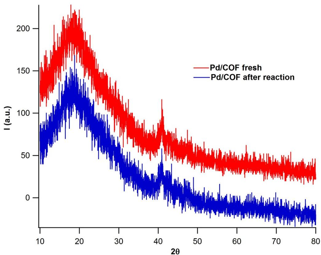
**Figure S2.** X-ray diffraction for Pd/COF fresh and spent catalysts
