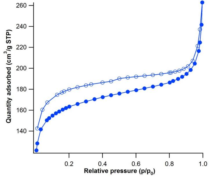
**Figure S3.** Nitrogen adsorption-desorption isotherms at -196 °C of spent Pd/COF.
