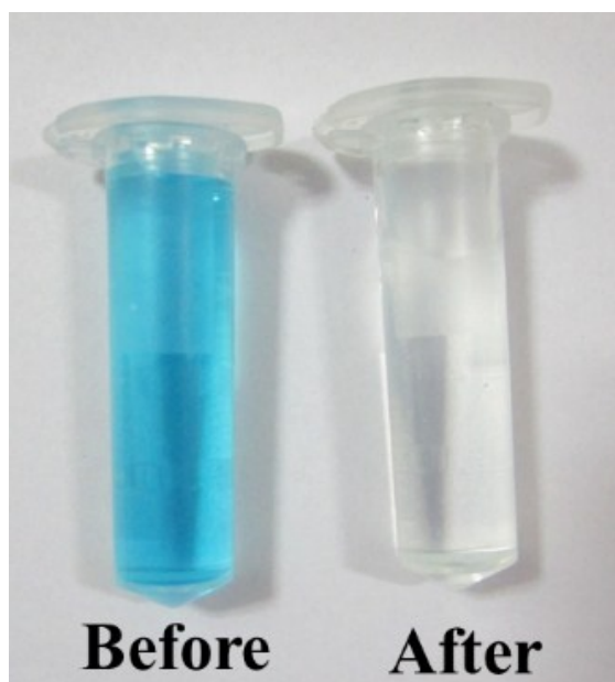
Fig. S7 Photographs of MB dye before and after the photocatalytic degradation using Au@Ag@TNF (S4) photocatalyst under solar light irradiation.
