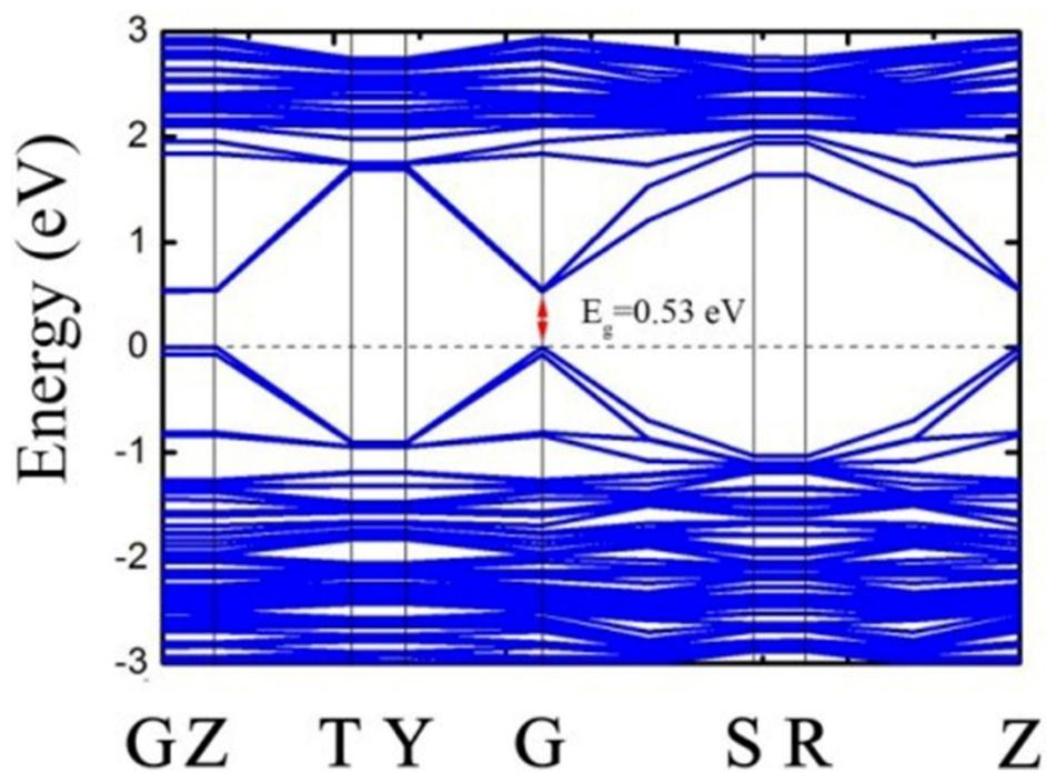
**Fig. S2** Band structures for TiO<sub>2</sub>/GR. The horizontal dashed line indicates the Fermi level.
