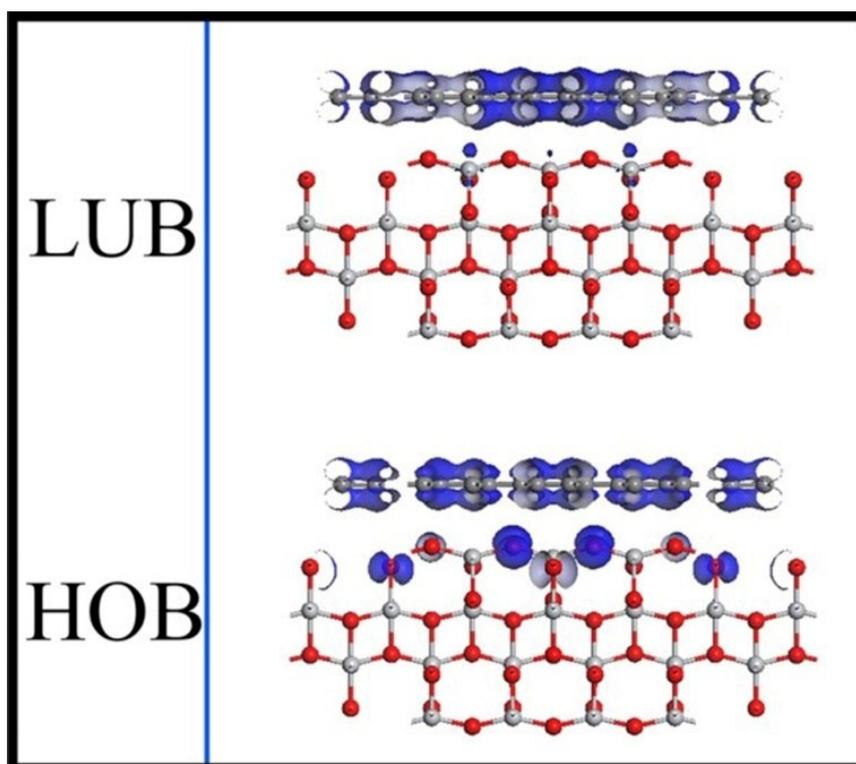
**Fig. S4** Maps of the electron and hole density distributions for the HOB and LUB with an isovalue of  $0.003 e/\text{\AA}^3$  for the hybrid TiO<sub>2</sub>/GR. Here, HOB and LUB denote the highest-occupied and lowest-unoccupied bands, respectively. A type-I heterojunction form on TiO<sub>2</sub>/GR nanocomposites.
