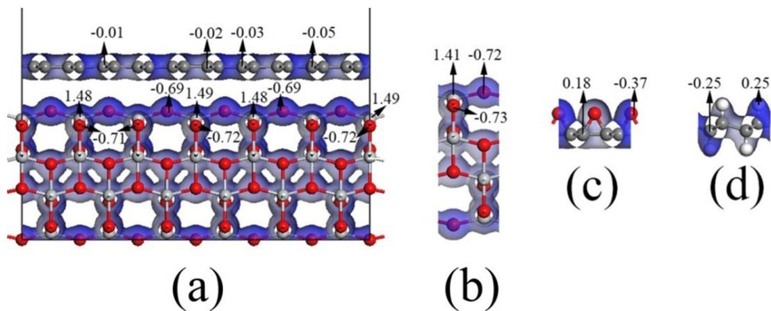
**Fig. S5** Charge distribution map of (a) TiO<sub>2</sub>/GR, (b) pure TiO<sub>2</sub>(001), (c) monolayer RGO and (d) monolayer GRH with a isovalue of 0.4 e/Å<sup>3</sup>. Light gray, red, black, and white sphere represent Ti, O, C and H atoms, respectively.
