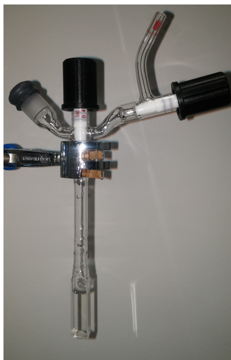
Fig. S5 Custom-made quartz cuvette fitted with high vacuum valves for use in the transient absorption experiments of AQN.
