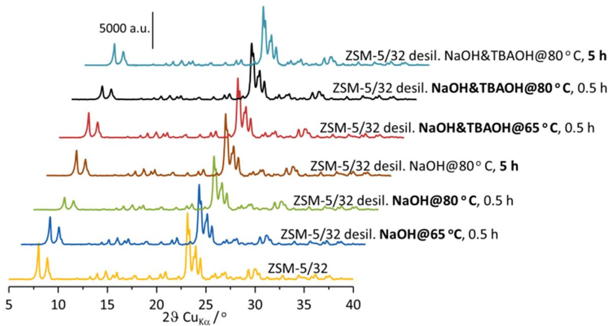
Figure SI.1. X-ray diffraction patterns of parent and desilicated ZSM-5 zeolites.
