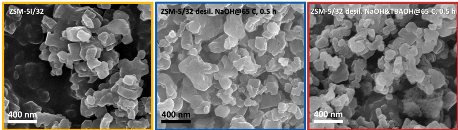
Figure SI.2. SEM images of the parent (left) and two representative samples treated with NaOH (middle) and NaOH&TBAOH (right), both treated at 65 °C, 0.5 h.
