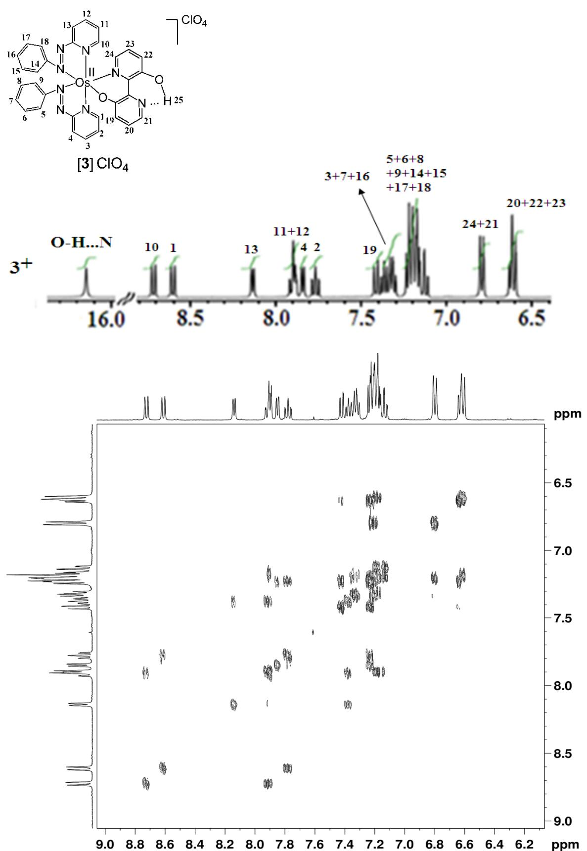
**Fig. S6**  $^1\text{H}$ -NMR and  $^1\text{H}$ - $^1\text{H}$  COSY NMR spectra of  $3^+$  (in  $\text{CD}_3\text{CN}$ ).
