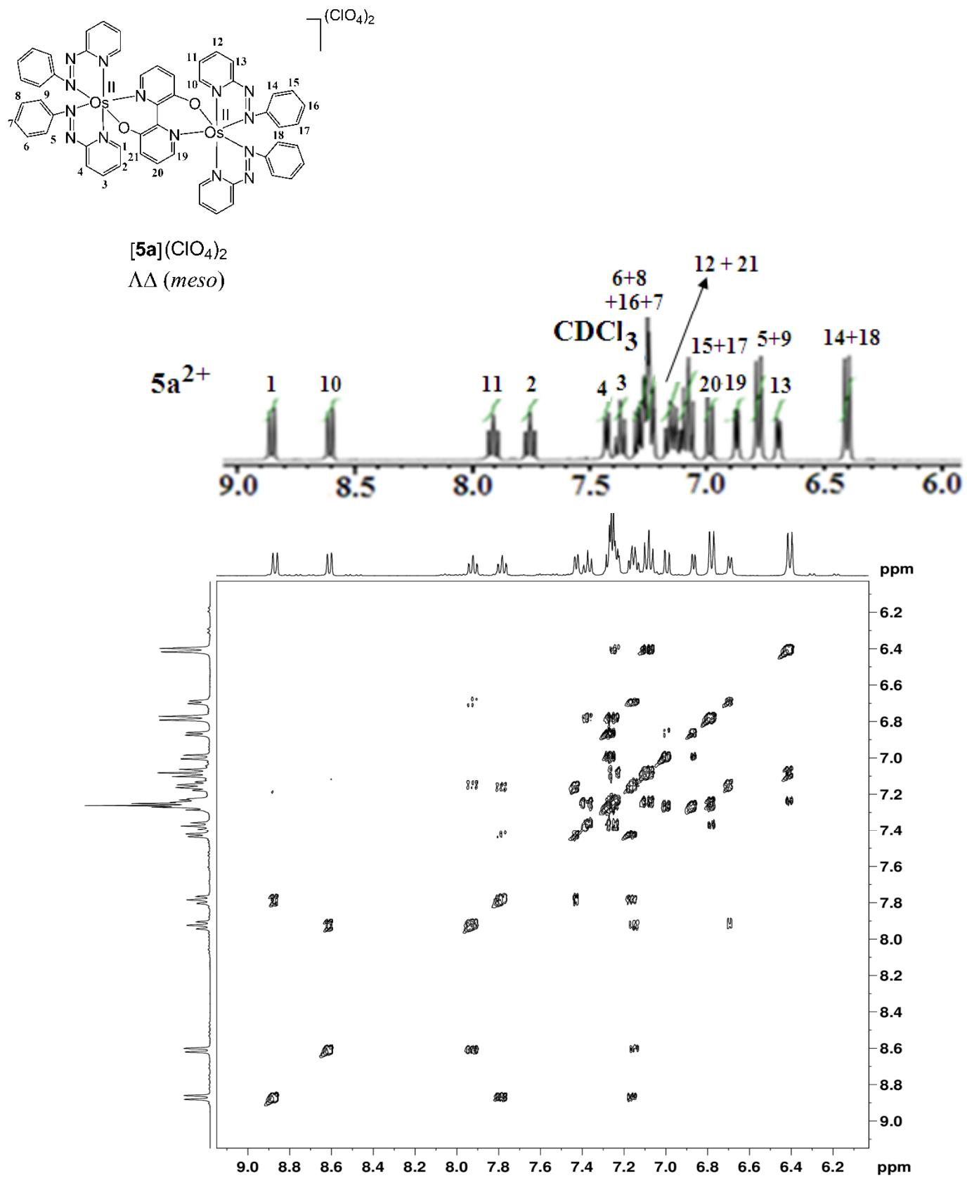
**Fig.S8**  $^1\text{H}$ -NMR and  $^1\text{H}$ - $^1\text{H}$  COSY NMR spectra of  $5a^{2+}$  (in  $\text{CDCl}_3$ ).
