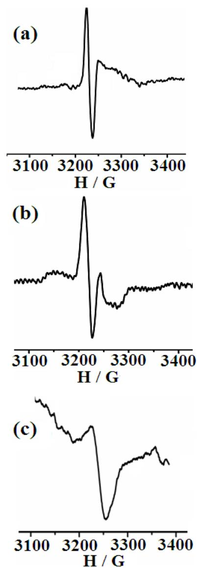
**Fig. S20** EPR spectra of coulometrically generated (a)  $\mathbf{2}^{2+}$ , (b)  $\mathbf{5a}^{3+}$  and (c)  $\mathbf{6}^+$ .
