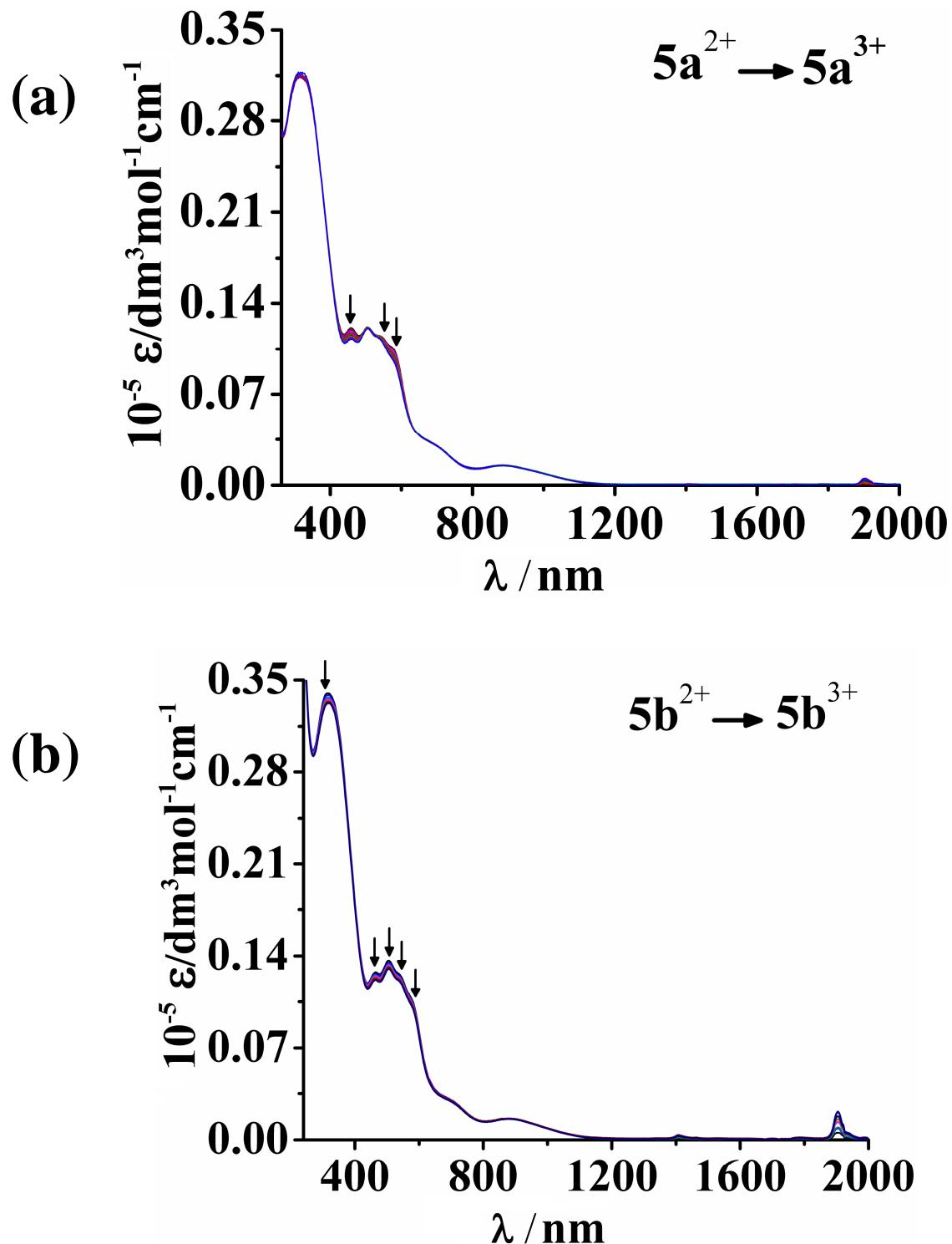
**Fig. S17** UV-vis-NIR spectroelectrochemical plots for the conversions of (a)  $5\mathbf{a}^{2+} \rightarrow 5\mathbf{a}^{3+}$  and (b)  $5\mathbf{b}^{2+} \rightarrow 5\mathbf{b}^{3+}$  ( $10^{-5}$  M) on sequential additions of  $(\text{NH}_4)_2\text{Ce}(\text{NO}_3)_6$  (CAN) ( $10^{-3}$  M) up to one equivalent in  $\text{CH}_3\text{CN}$ .
