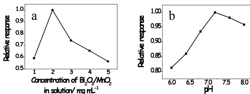
Fig. S8: Effect of (a) concentration of BM NFs in solution and (b) pH of electrolyte on the amperometric response of BM NFs/Nf/GCE to  $5 \mu\text{M H}_2\text{O}_2$ .
