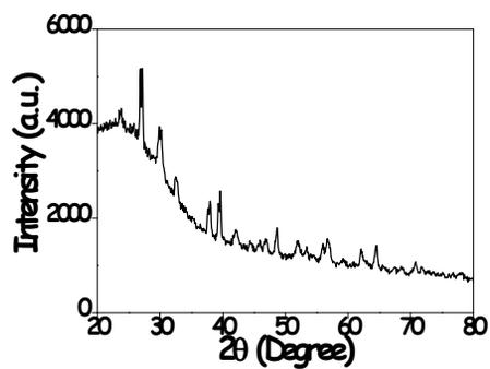
Fig. S4: XRD pattern of as-synthesized  $\text{Bi}(0)$  nanoparticles.
