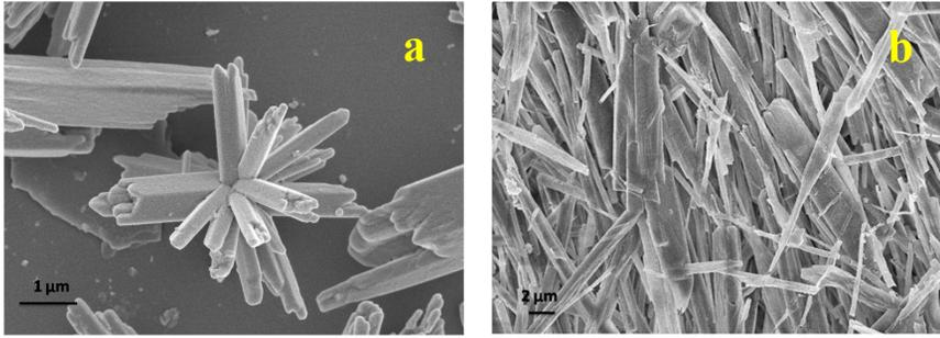
Fig. S1: FESEM images of (a)  $\text{Bi}_2\text{O}_3$  and (b)  $\text{MnO}_2$ .
