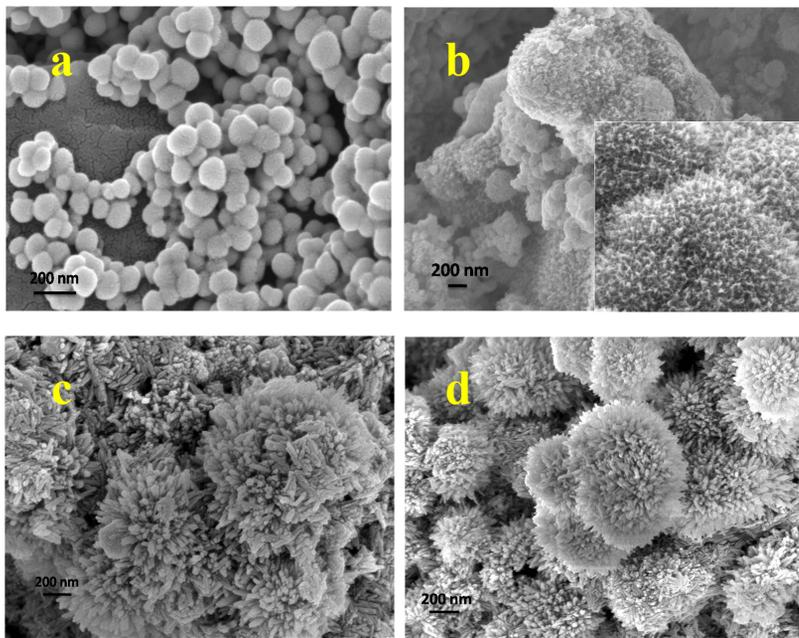
Fig. S2: Time dependent synthesis of  $\text{Bi}_2\text{O}_3/\text{MnO}_2$  NFs at (a) 1 h, (b) 5 h, (c) 9 h and (d) 12 h.
