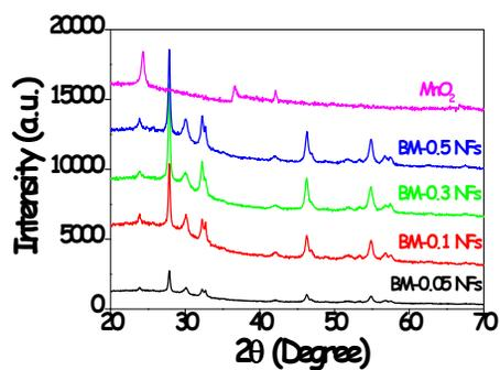
Fig. S6: Comparative XRD pattern of as-synthesized various BM NFs composites and  $\text{MnO}_2$ .
