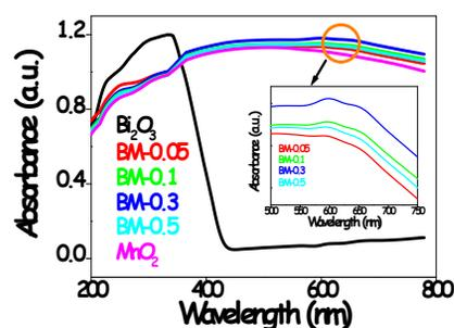
Fig. S7: (a) UV-Vis diffuse reflection spectra of the as-prepared various  $\text{Bi}_2\text{O}_3/\text{MnO}_2$ , bare  $\text{Bi}_2\text{O}_3$  and  $\text{MnO}_2$  samples and inset shows enlarged view of various  $\text{Bi}_2\text{O}_3/\text{MnO}_2$  composites.
