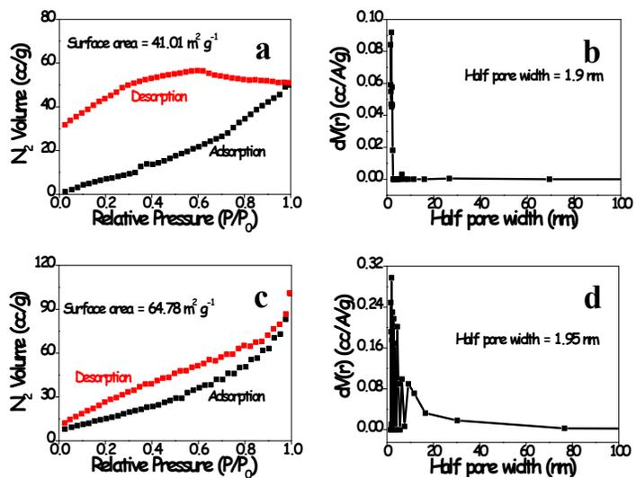
Fig. S3: (a, c) Nitrogen adsorption and desorption isotherm and (b, d) pore size distribution plot of  $\text{Bi}_2\text{O}_3$  and  $\text{MnO}_2$  materials respectively.
