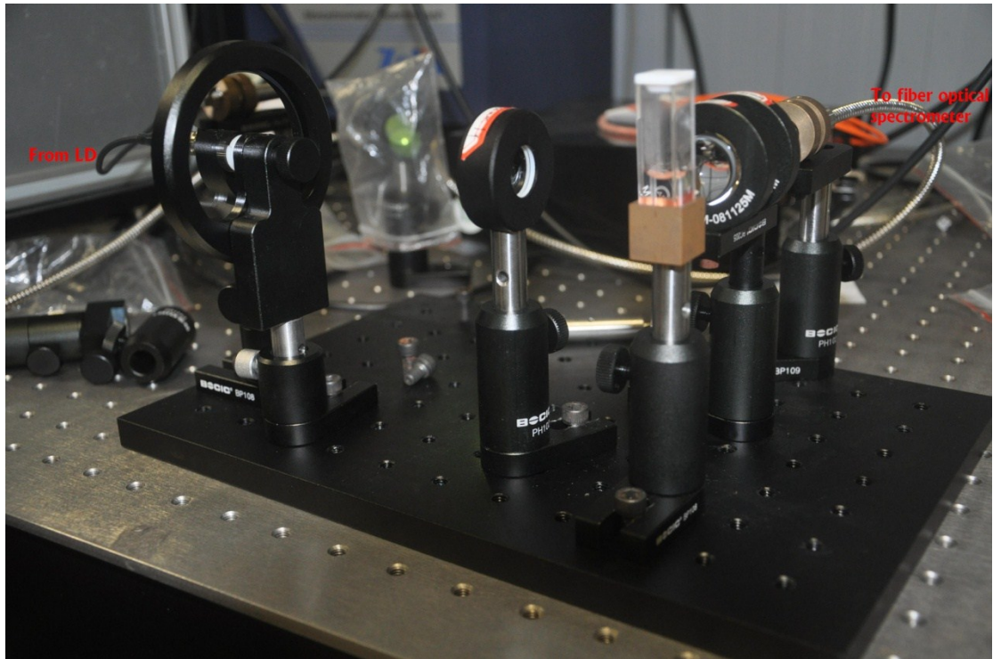
Figure S1. Optical path image of spectroscopic UCL measurement
