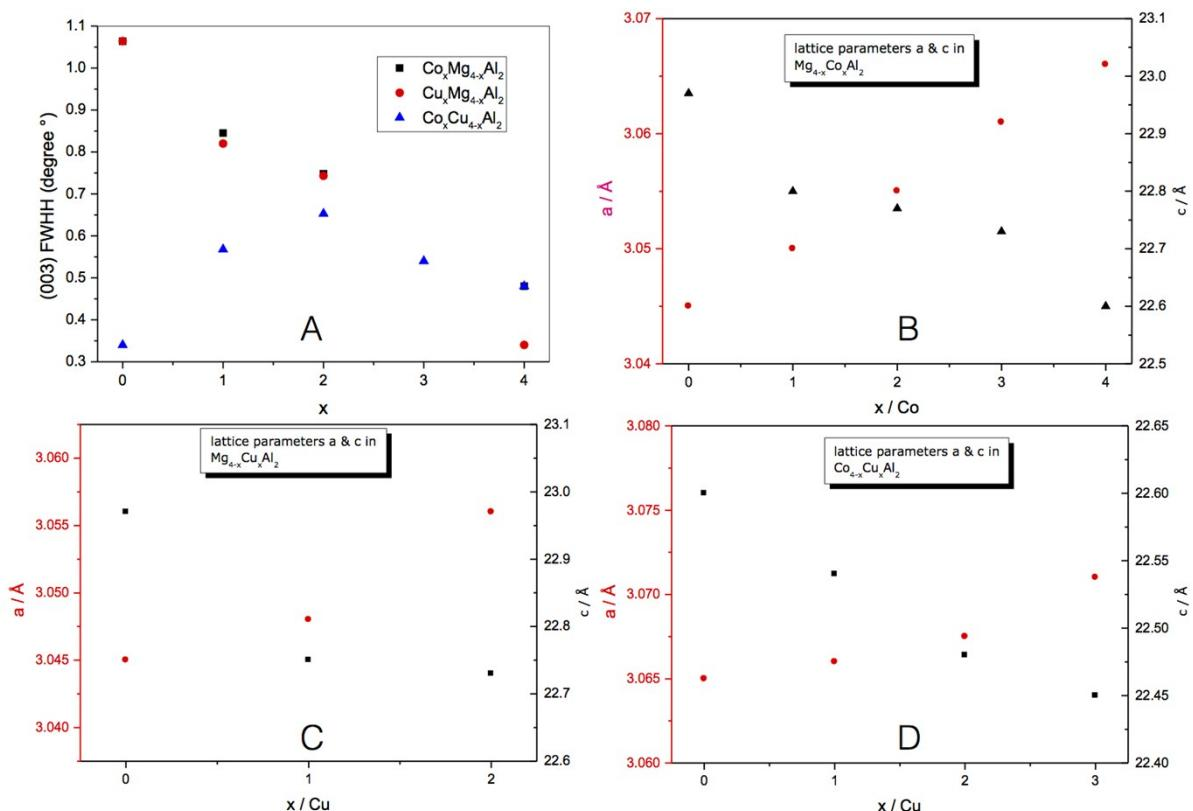
Fig. S1. Extracted data from XRD diffractograms: A) Evolution of Full Width at Half Height of the (003) reflection as function of the metal substitution; Evolution of lattice parameters a, c for B) MgCoAl, C) MgCuAl and D) CoCuAl.
