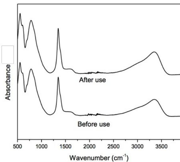
Fig. S6. FT-IR spectra of  $\text{Co}_3\text{Cu}_1\text{Al}_2$  before / after orange II degradation.
