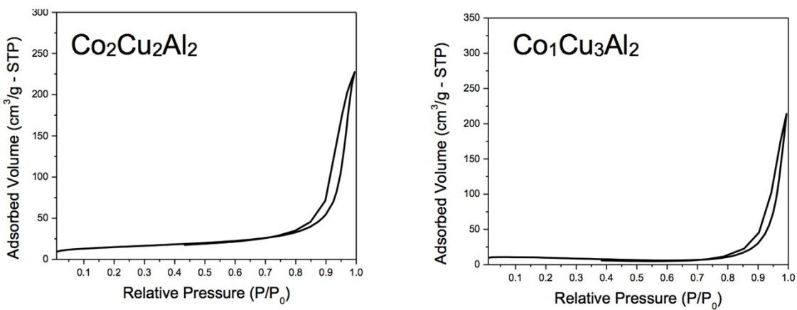
Fig. S2. N<sub>2</sub> adsorption-desorption isotherms of LDH materials
