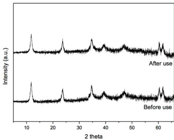
Fig. S5. XRD of  $\text{Co}_3\text{Cu}_1\text{Al}_2$  before / after orange II degradation.
