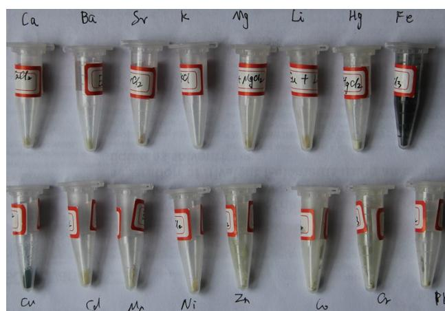
**Fig. S3** Photos of  $\mathbf{M}^{n+}@\mathbf{Eu-CP}$  samples after immersing in metal ion solutions.
