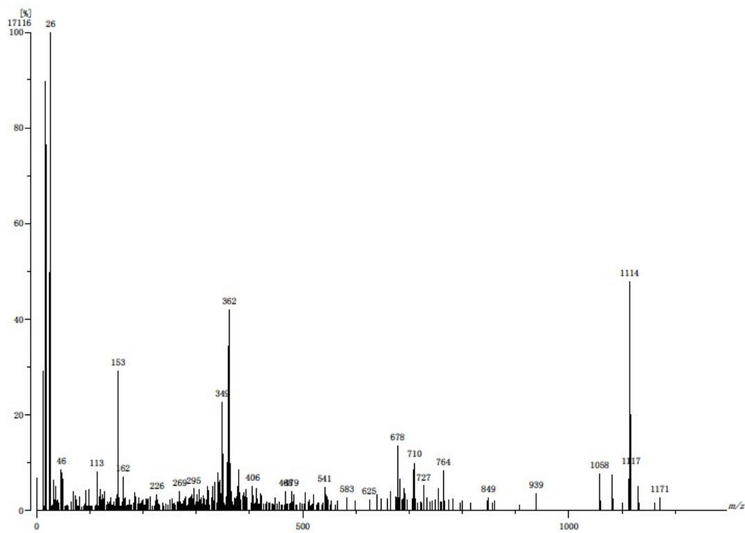
**Figure S2.** FAB<sup>-</sup> MS of **1<sup>THF</sup>**.
