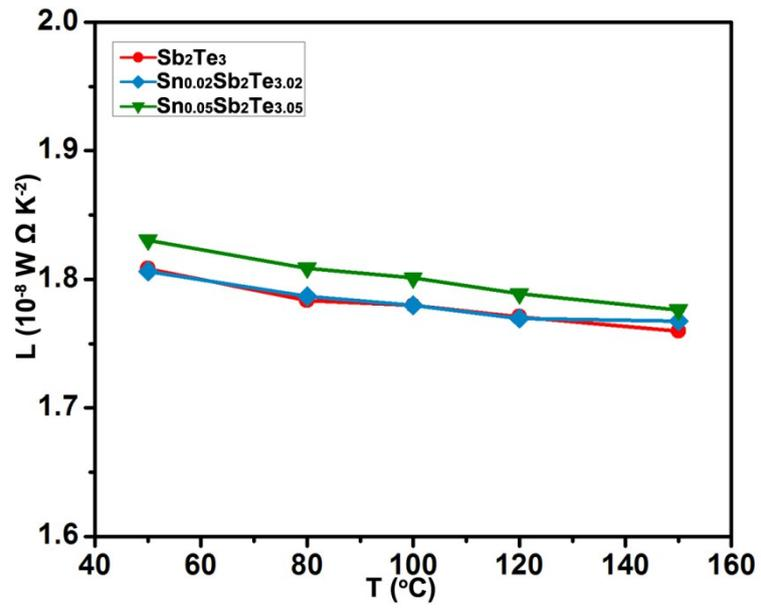
**Fig. S6** The calculated Lorenz number ( $L$ ) of  $\text{Sb}_2\text{Te}_3$  and  $\text{Sn}_x\text{Sb}_2\text{Te}_{3+x}$  ( $x = 0.02$  and  $0.05$ ) samples.
