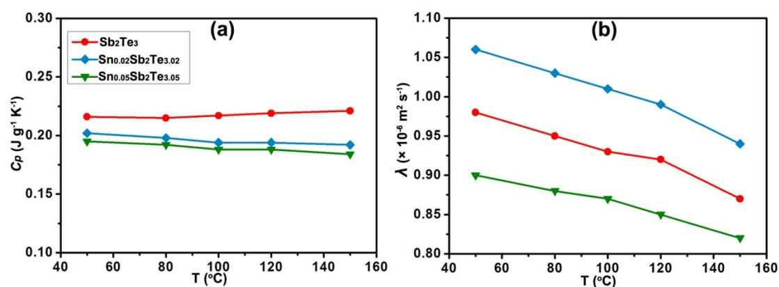
**Fig. S5** The measured specific heat ( $C_p$ ) and thermal diffusivity ( $\lambda$ ) of  $\text{Sb}_2\text{Te}_3$  and  $\text{Sn}_x\text{Sb}_2\text{Te}_{3+x}$  ( $x = 0.02$  and  $0.05$ ) samples: (a)  $C_p$ ; (b)  $\lambda$ .
