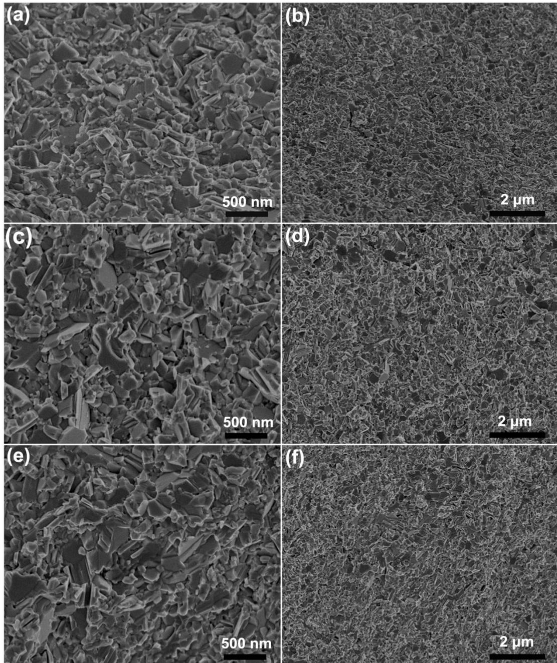
**Fig. S3** SEM images of the as-sintered  $\text{Sb}_2\text{Te}_3$  (a,b),  $\text{Sn}_{0.02}\text{Sb}_2\text{Te}_{3.02}$  (c,d) and  $\text{Sn}_{0.05}\text{Sb}_2\text{Te}_{3.05}$  (e,f) bulk samples.
