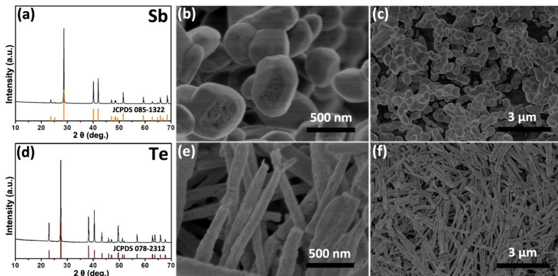
**Fig. S1** XRD patterns and SEM images of as-synthesized elemental Sb and Te precursors: (a,b,c) Sb; (d,e,f) Te. The orange and wine bars stand for the standard XRD pattern of Sb (JCPDS 085-1322) and Te (JCPDS 078-2312), respectively.
