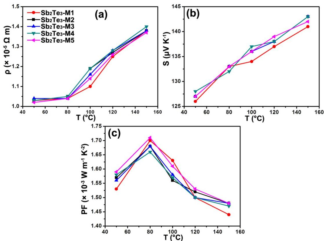
**Fig. S4** The repeated measurement of temperature dependent resistivity (a) and Seebeck coefficient (b) and calculated power factor (c) on the  $\text{Sb}_2\text{Te}_3$  nanobulk sample.
