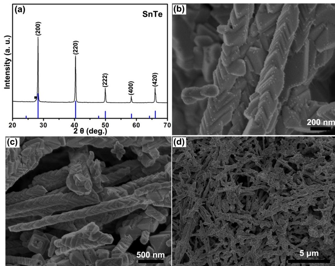
**Fig. S2** (a) XRD pattern of the SnTe powder synthesized at 120 °C for 24 h. The blue bars stand for the standard XRD pattern of SnTe (JCPDS 065-7162) and the black solid square (■) stands for Te. (b–d) SEM images of as-synthesized SnTe powder.
