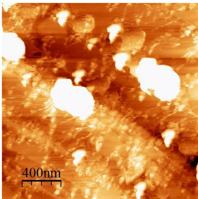
**Figure S2.** AFM topography-image of 2x2 μm area of large aggregates palladium on a HOPG surface
