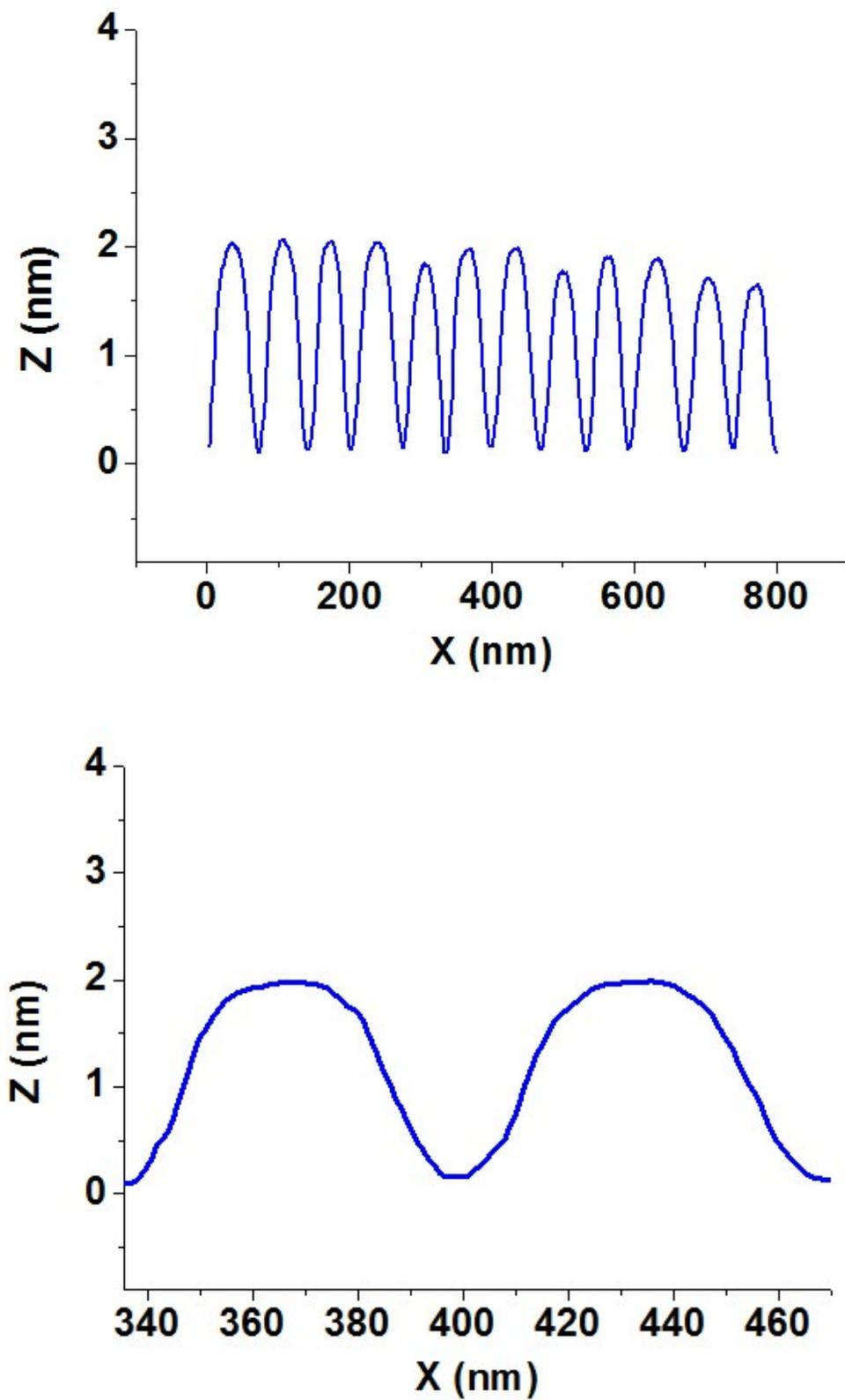
**Figure S8.** Profile of palladium bands along the black line (Fig.4 in article) after deconvolution procedure (radius of the tip is 10 nm). Platform between the bands have a width of 3-4 nm
