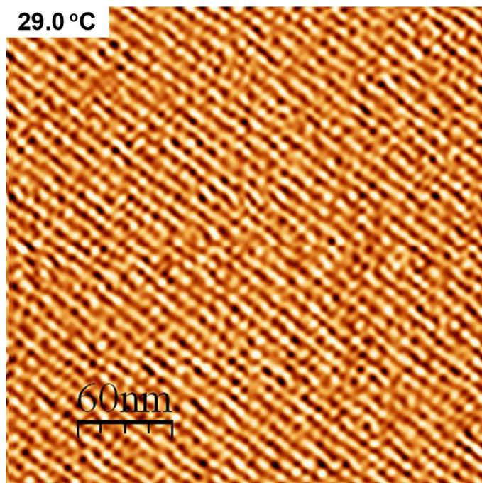
**Figure S5.** AFM image (300×300 nm) of adsorbed structure of CTAB at the graphite-water interface (t = 29.0 °C)
