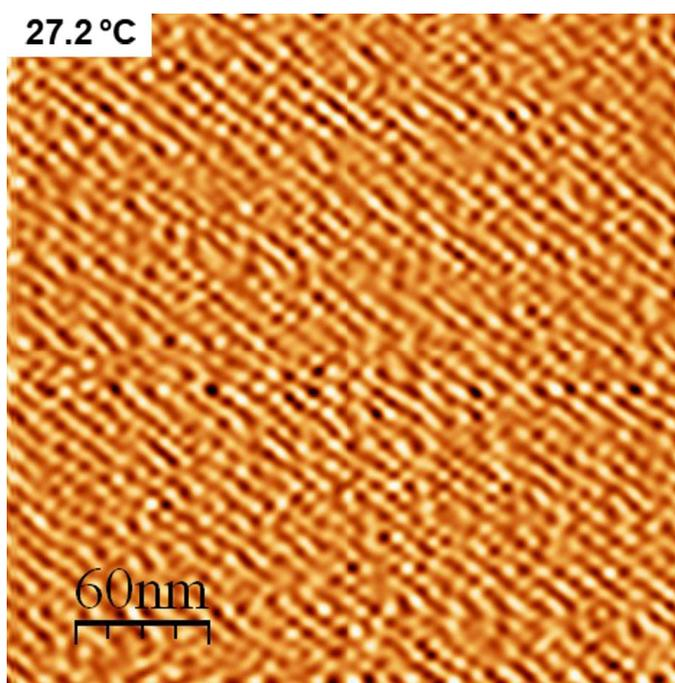
**Figure S4.** AFM image (300×300 nm) of adsorbed structure of CTAB at the graphite-water interface (t = 27.2 °C)
