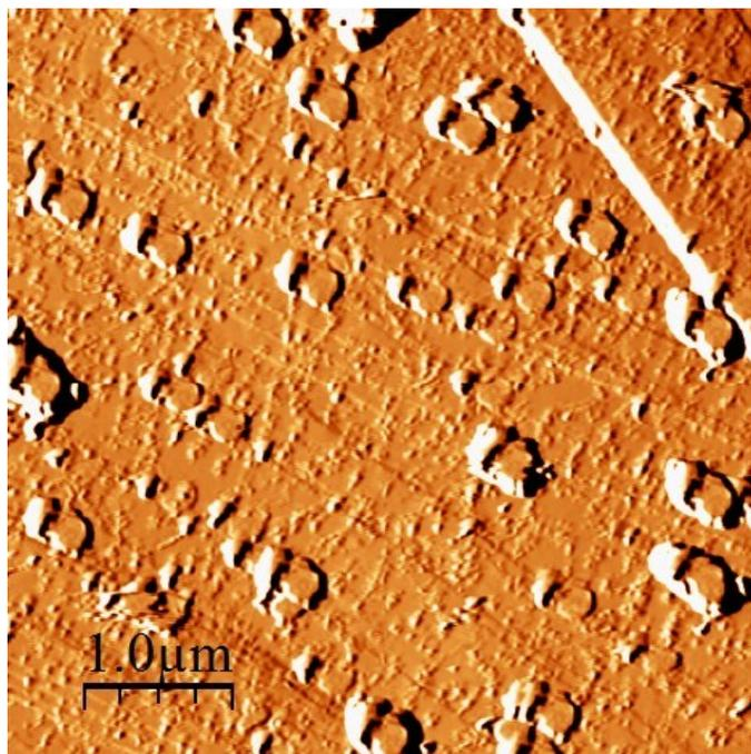
**Figure S3.** AFM image of a large aggregate and palladium bands on a HOPG surface
