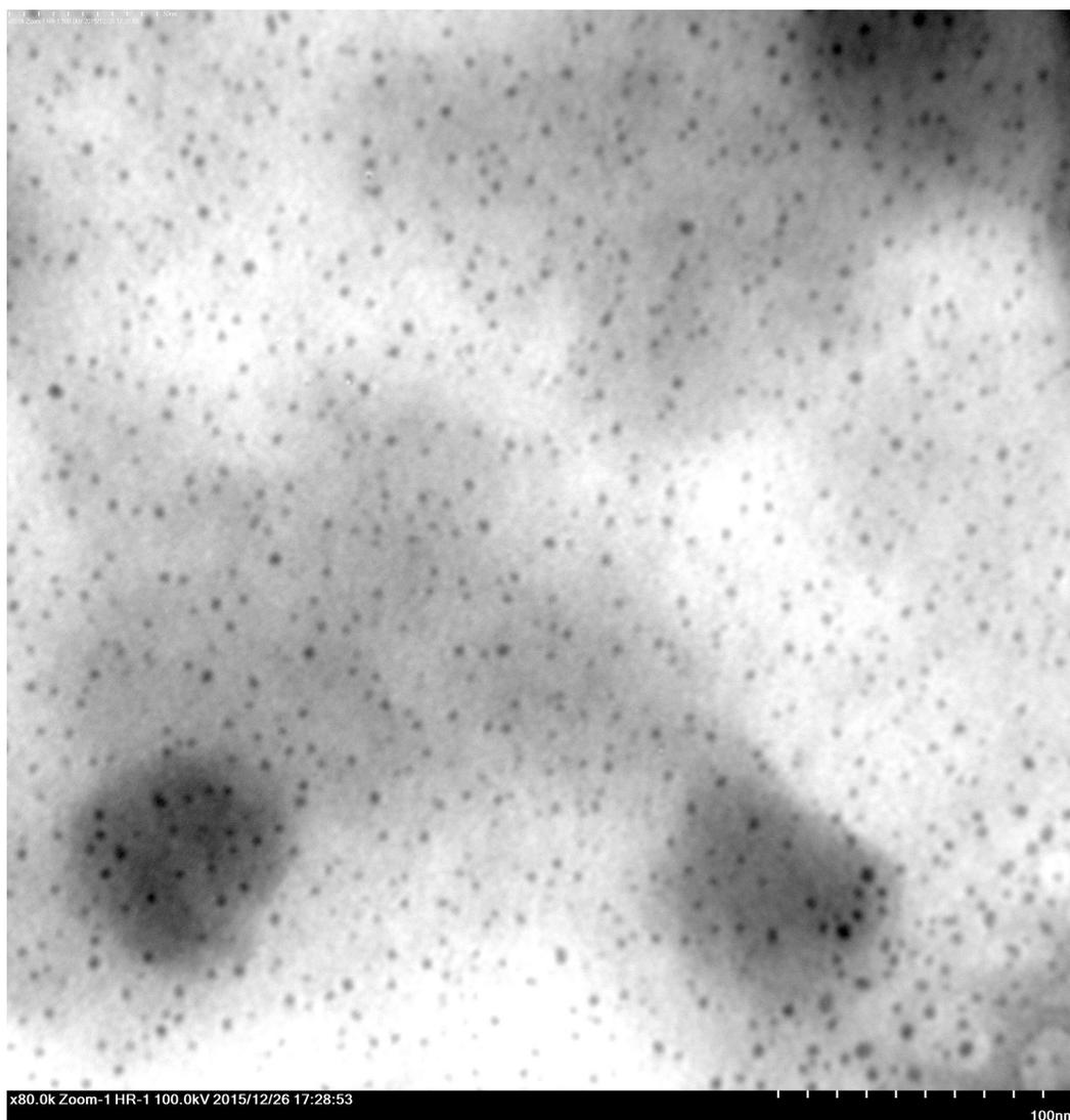
**Fig. S10.** TEM image of Pd particles deposited on the surface of formvar using CTAB micellar template.
