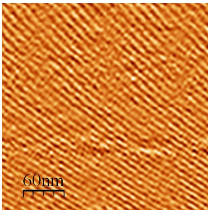
**Figure S6.** AFM image (300×300 nm) of adsorbed structure of CTAB at the graphite-water interface, from bottom of image to its top temperature is changed (28.2-28.4 °C)
