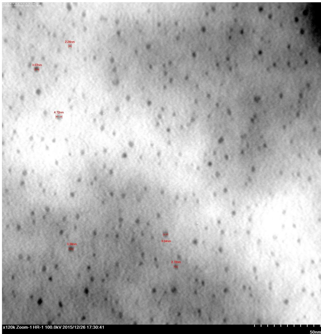
**Fig. S9.** TEM image of Pd particles deposited on the surface of formvar using CTAB micellar template
