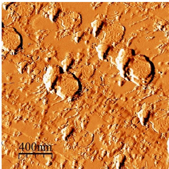
**Figure S1.** AFM image of 2x2 μm area of large aggregates palladium on a HOPG surface
