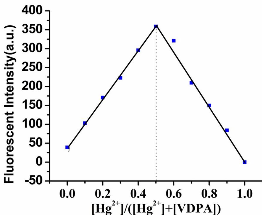
Fig S5. Job's plot for the binding of **VDPA** with  $\text{Hg}^{2+}$ , the total concentration of **VDPA** and  $\text{Hg}^{2+}$  is  $20\ \mu\text{M}$ .
