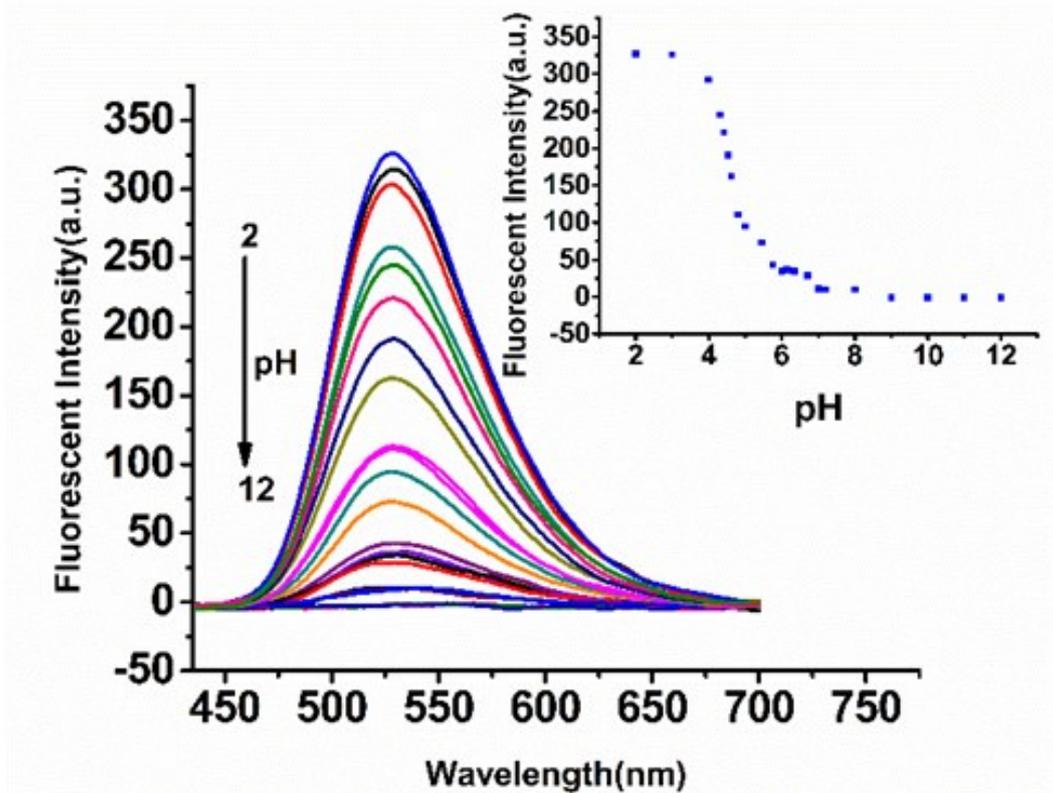
Fig S6. Fluorescence pH titration spectra of VDPA (adjusted by 1 M HCl or 1 M NaOH) in water solution. Inset: Fluorescence intensity changes of VDPA under different pH,  $\lambda_{\text{ex}} = 400 \text{ nm}$ ,  $\lambda_{\text{em}} = 540 \text{ nm}$ , 25 °C, water).
