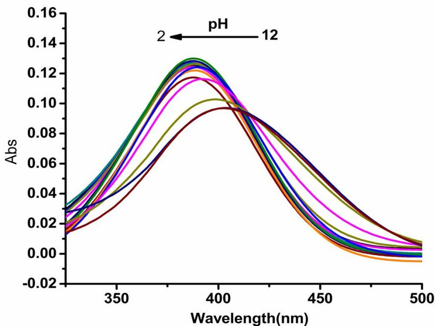
Fig S7. The absorption properties of VDPA on changing the pH
