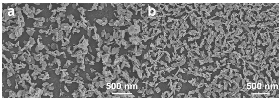
**Fig. S3** SEM images of synthesized Gd-CPs with addition of TEA in DMF/water mixture: a) CP-5; b) CP-6 (Table 1).
