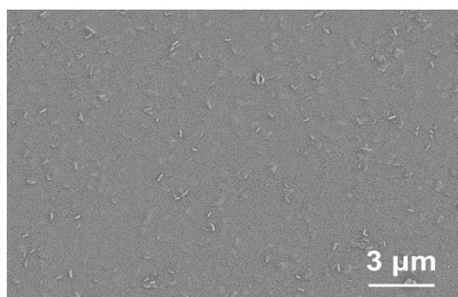
**Fig. S10** SEM image of the surface of the Tb-CP/MC composite film.
