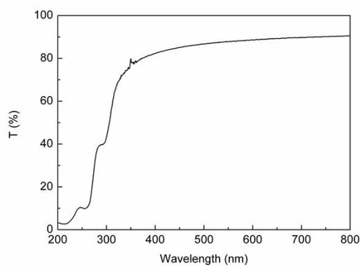
**Fig. S11** Transmittance of the composite film. No scattering is found between 350 and 800 nm. Considering the particle sizes around 250 nm, we conclude no obvious particle aggregation in the film.
