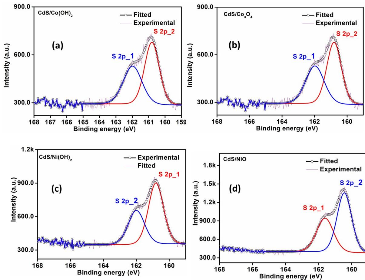
**Figure SI 5** XPS spectra of S 2p of (a) CdS/Co(OH)<sub>2</sub> (b) CdS/Co<sub>3</sub>O<sub>4</sub> (c) CdS/Ni(OH)<sub>2</sub> (d) CdS/NiO electrodes before PEC measurements.
