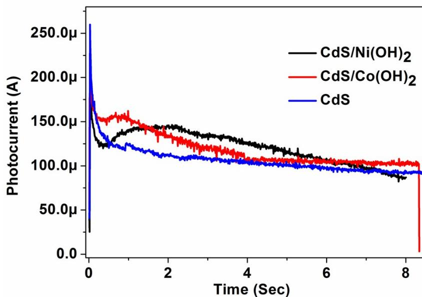
**Figure SI 4** Comparison of time dependent chronoamperometric measurement of *M*-OH modified CdS photoanodes
