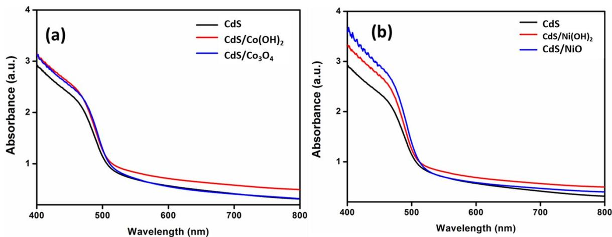
**Figure SI 6** Absorption spectra of (a) Co(OH)<sub>2</sub> and Co<sub>3</sub>O<sub>4</sub> modified CdS thin films (b) Ni(OH)<sub>2</sub> and NiO modified CdS thin films.
