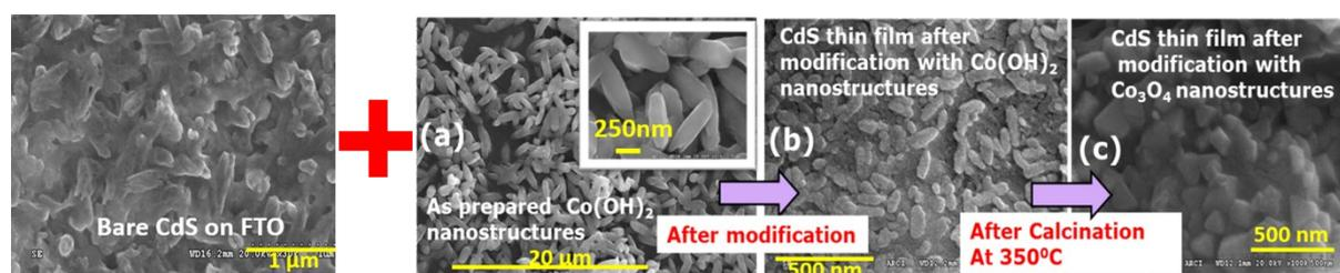
**Figure SI 1.** FESEM of (a) As synthesized  $\text{Co}(\text{OH})_2$  nano-rice structures; And CdS thin films modified with (b)  $\text{Co}(\text{OH})_2$ ; (c)  $\text{Co}_3\text{O}_4$ .
