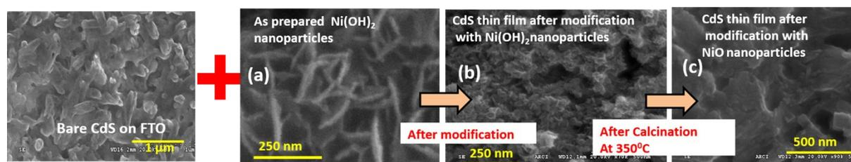
**Figure SI 2** (a) SEM of (a) As synthesized  $\text{Ni}(\text{OH})_2$  nano-sheets structures; And CdS thin films modified with (b)  $\text{Ni}(\text{OH})_2$ ; (c)  $\text{NiO}$ .
