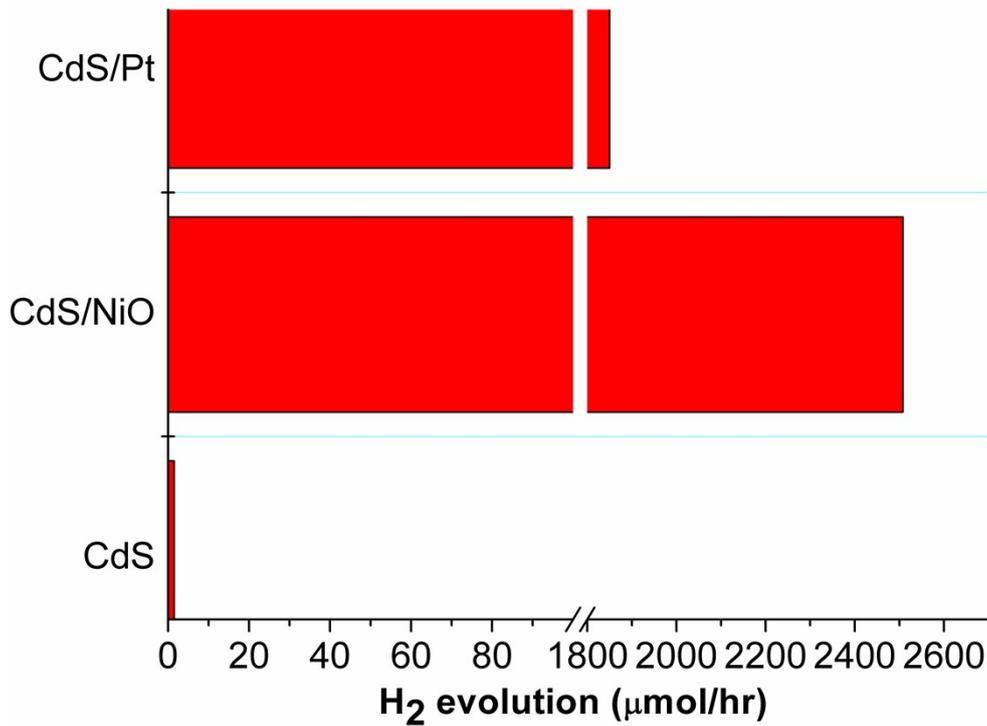
**Figure SI 7.** Hydrogen evolution rates of CdS, CdS/NiO and CdS/Pt.
