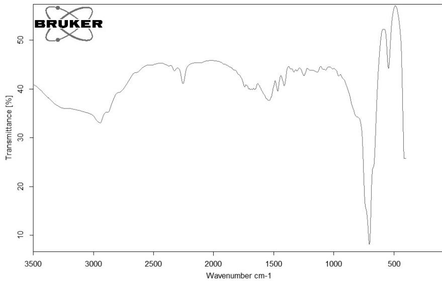
Figure S28. IR spectrum of  $[\text{Me}_2\text{HNCH}_2\text{CNH}][\text{AsF}_6]_2$ .
