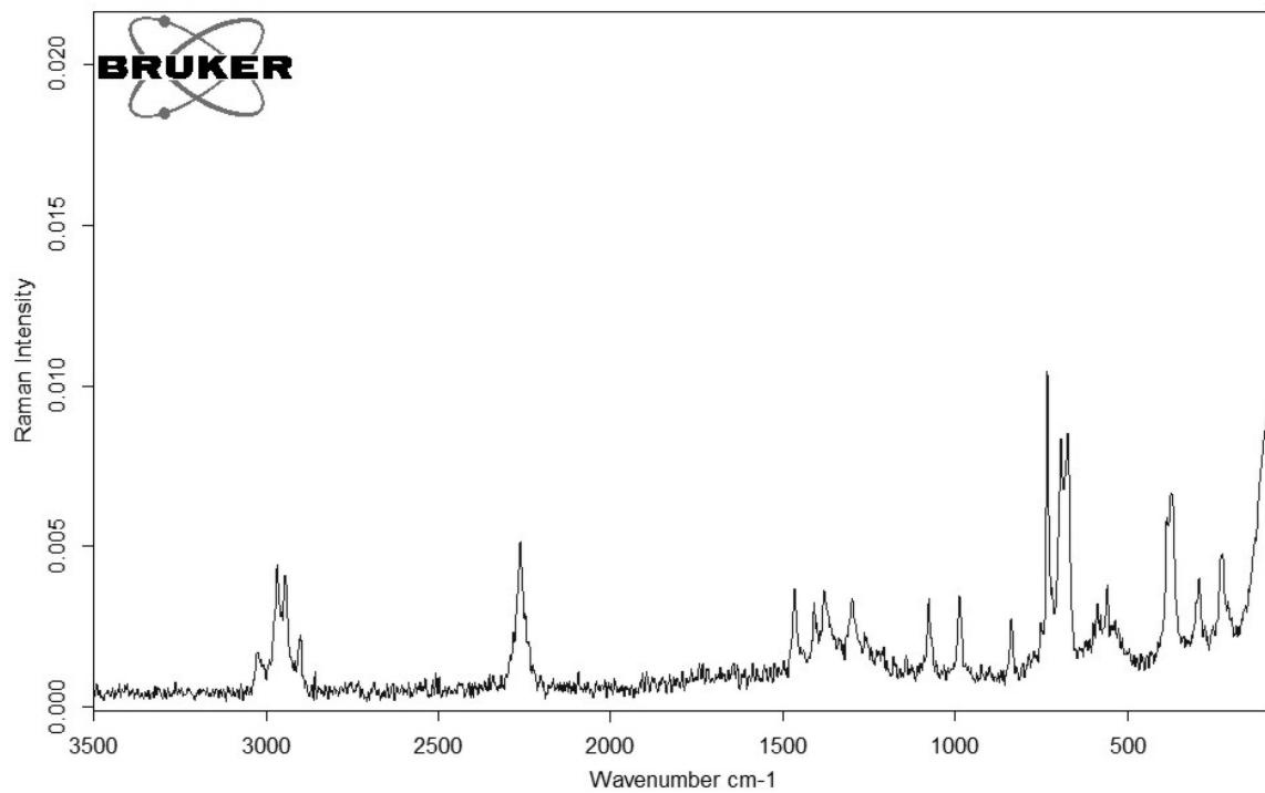
Figure S19. Raman spectrum of  $[\text{C}_2\text{H}_5\text{CNH}][\text{AsF}_6]$ .
