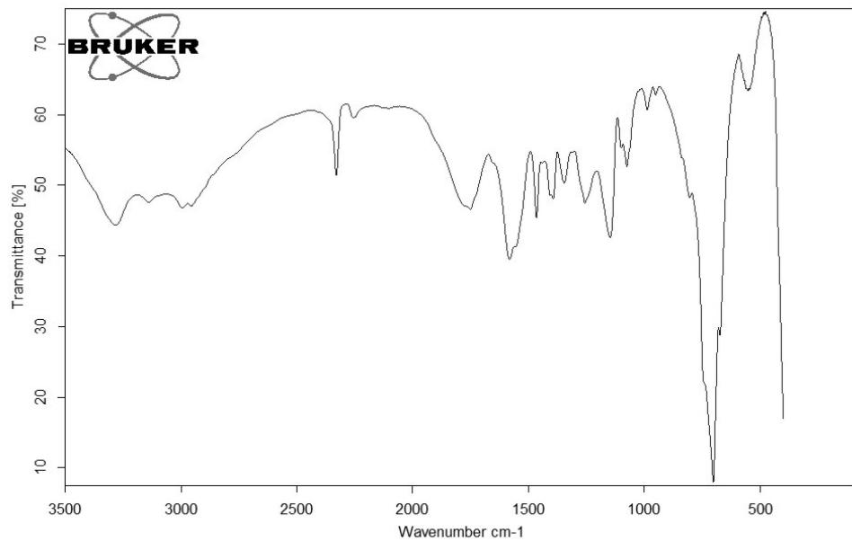
Figure S25. IR spectrum of  $[\text{C}_2\text{H}_5\text{CNH}][\text{AsF}_6]$ .
