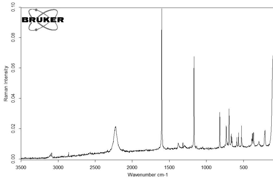
Figure S22. Raman spectrum of  $[p\text{-C}_6\text{H}_4(\text{CNH})_2]\text{[AsF}_6\text{]}_2$ .
