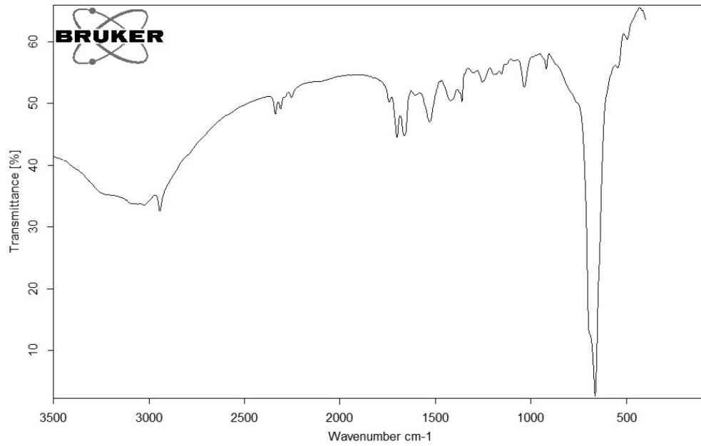
Figure S24. IR spectrum of  $[\text{CH}_3\text{CNH}][\text{Sb}_2\text{F}_{11}]$ .
