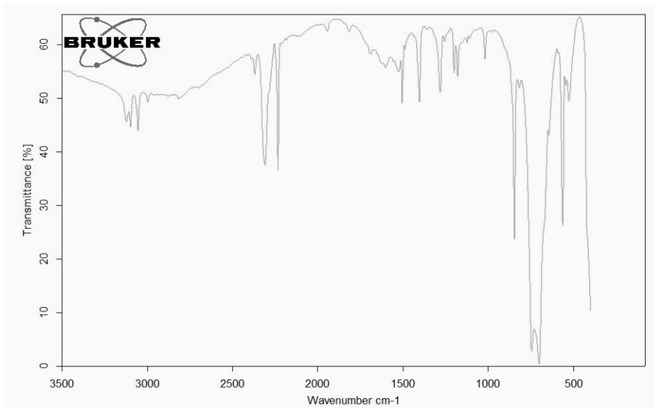
Figure S30. IR spectrum of  $[p\text{-C}_6\text{H}_4(\text{CNH})_2][\text{AsF}_6]_2$ .
