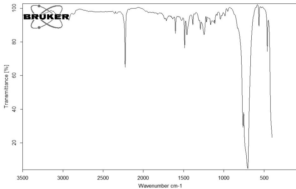
Figure S29. IR spectrum of  $[o\text{-CH}_3\text{C}_6\text{H}_4\text{CNH}][\text{AsF}_6]$ .
